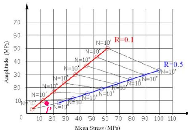
Fig. 2. GD-diagram of the SCWTBs with material partial safety factor 5.0
