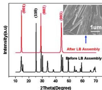
Fig.4: XRD patterns of  $\text{VO}_2$  nanowires before and after LB assembly, insert is SEM image of  $\text{VO}_2$  nanowire LB film.<sup>[5]</sup>
