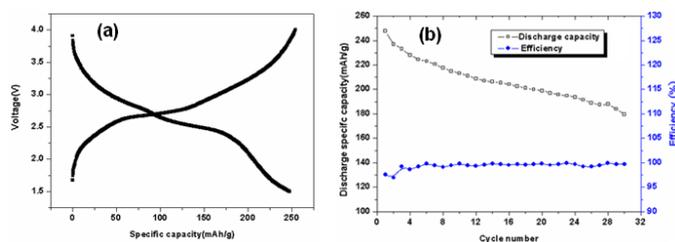
Fig.3: Initial charge/discharge curve of VO<sub>2</sub>(B) nanorods(a), the curves of discharge specific capacity and efficiency vs. cycling number (b).<sup>[4]</sup>
