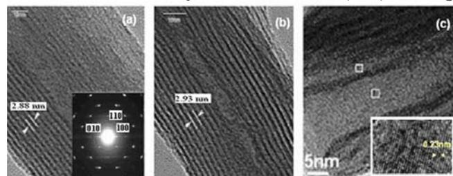
Fig.1: The HRTEM images of VONT (a), V<sub>0.99</sub>Mo<sub>0.01</sub>ONT (b), Ag-containing VONT (c).<sup>[3]</sup>
