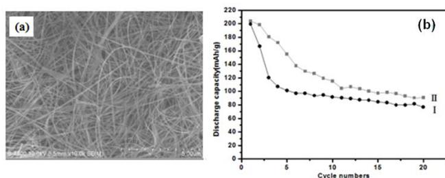
Fig.5: (a) Typical FE-SEM image of the  $\beta$ - $\text{AgVO}_3$  nanowires, (b) cyclability of the batteries assembled with the  $\beta$ - $\text{AgVO}_3$  nanowires ( I ) and the  $\text{AgVO}_3$ -PPy nanocables(II).<sup>[12]</sup>
