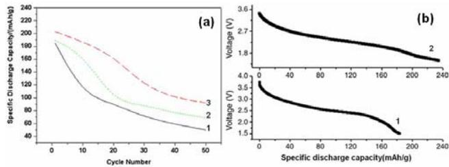
Fig.2: (a) The specific discharge capacity of VONT (1),  $V_{0.99}Mo_{0.01}$ ONT (2) and heated  $V_{0.99}Mo_{0.01}$ ONT (3), (b) first discharge cure of pure (1) and Ag-containing (2) VONTs.<sup>[3]</sup>
