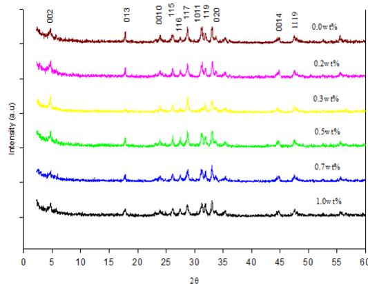
Figure 2. XRD pattern for pure and nano- $\gamma$ - $\text{Al}_2\text{O}_3$  added into BSCCO-2223 samples sintered at 24 hours
