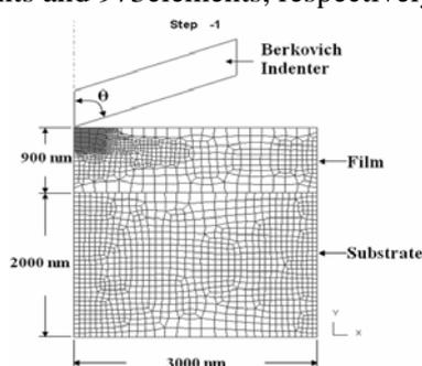
Fig. 1. FEM model of film-substrate system
