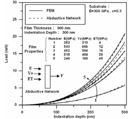
Fig. 4 Comparison between FEM and Abductive networks prediction for indentation load
