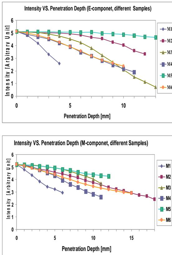
Fig. 1 Effective attenuations of the electric and magnetic fields of six groups of MWNT composite samples with the same (7 %) MWNT blend in composites. The frequency of the microwave signal is 9.968 GHz.
