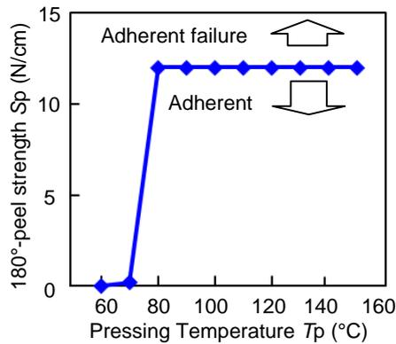
Fig.2 180°-peel strength  $S_p$  as a function of pressing temperature  $T_p$  for the bonded glass and irradiated PET film.
