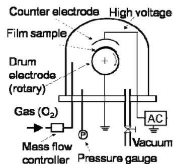
Fig. 1 Plasma irradiation system. Sample film is attached on the rotating drum electrode. Plasma is generated between the drum and counter electrodes.
