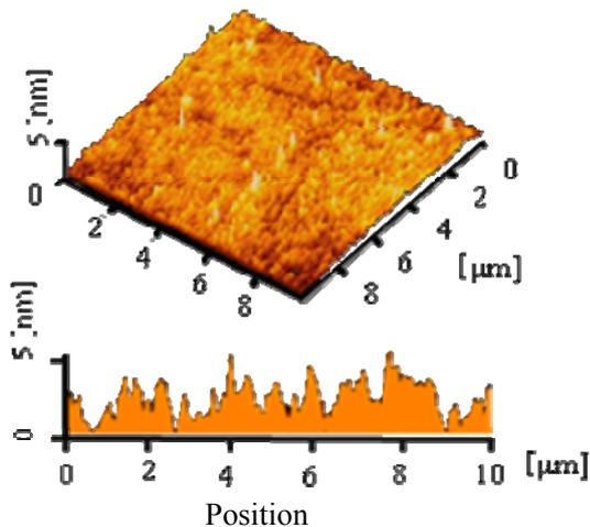
Fig. 3 AFM surface images (upper) and sectional profile (lower) for the used glass sample ( $R_a=0.22$  nm).
