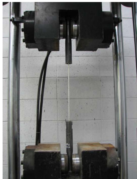
**Fig. 1** Tensile test of the GFRP rebar
