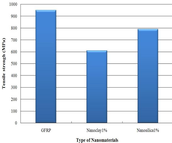
**Fig. 2** Tensile strength of the nano-GFRP bars
