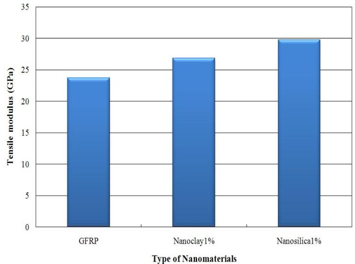
**Fig. 4** Tensile modulus of the nano-GFRP bars
