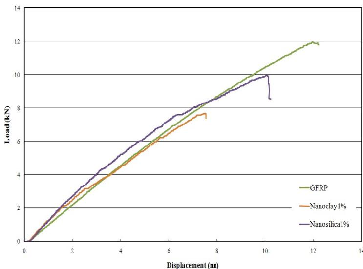
**Fig. 3** Load-displacement curves of the nano-GFRP bars
