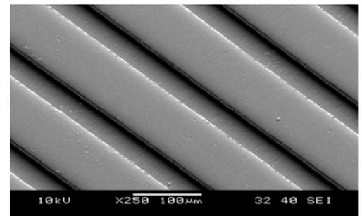
Fig. 4 SEM image of embossed microchannels at optimized parameters
