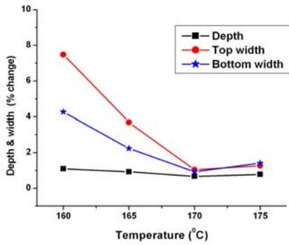
Fig. 1 Effect of embossing temperature on channel depth & width
