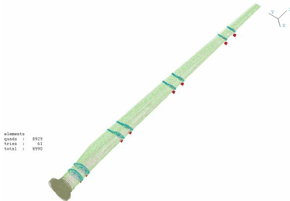
Figure 1 Blade FE model in GENESIS
