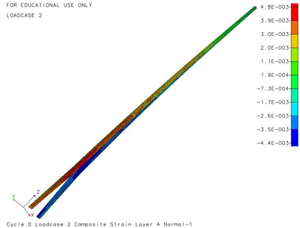
Figure 4 Spar cap composite strain in fiber direction
