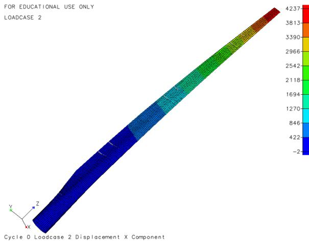
Figure 3 Maximum tip out of plane deflection, mm
