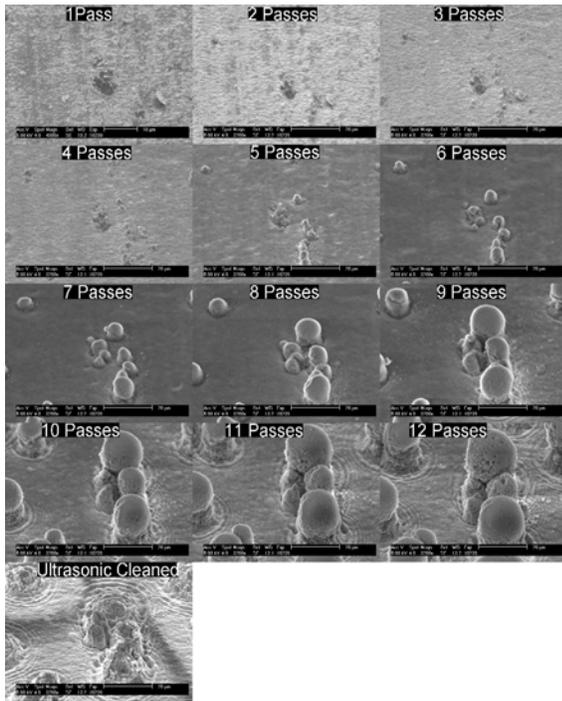
Fig. 3 Progressive set of SEM images showing the growth of each shell of the composite.
