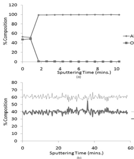
Fig. 4. Auger plots of elemental composition for (a) an unablated sample (b) a sample covered in aggregates.
