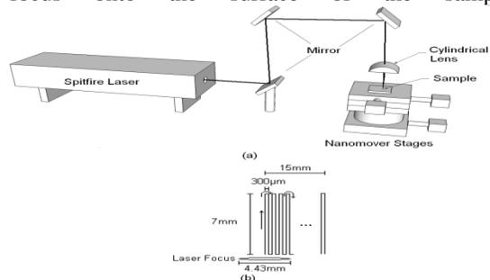
Fig. 1. (a). Experimental setup used in growing layered shelled nanocomposites and the blackening
