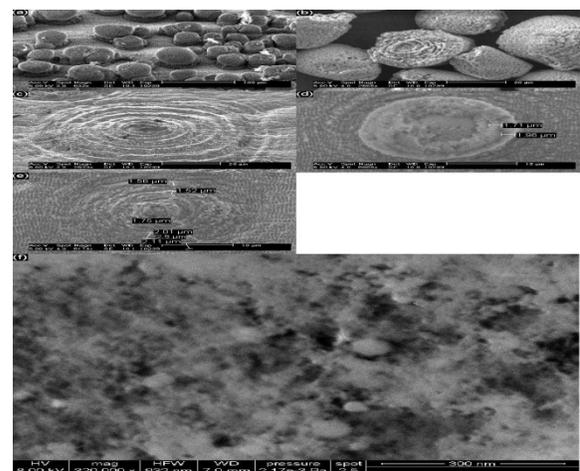
Fig. 2 (a) Spherical aggregates on 2024 T3 aluminum surface. (b) Aggregates that have been removed in an ultrasonic cleaner. (c) Ring structure that has developed under an aggregate. (d) An aggregate with several shells broken open. (e) Image of the ring structure left behind from the aggregate in (d). (f) A high magnification view of the inside of one of the aggregates.
