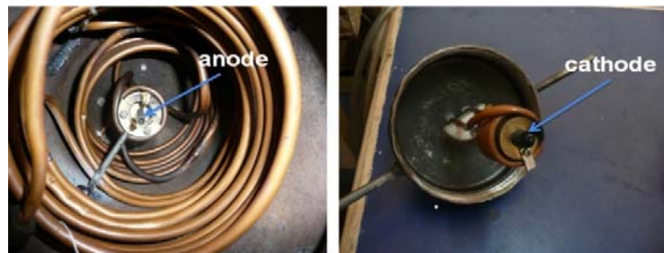
Fig-3: Anode, Cathode and the copper tubing
