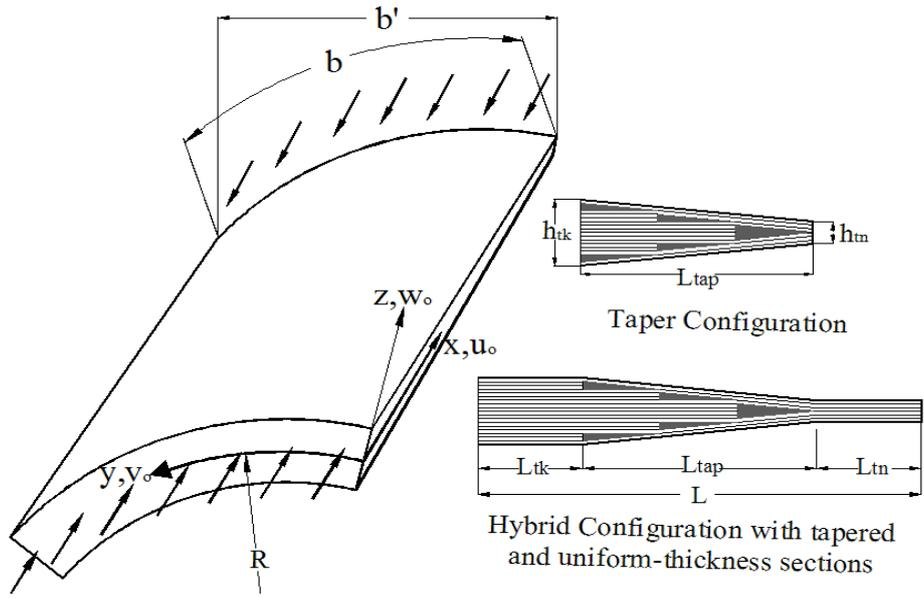
Figure 1: Different sections of curved laminated plate.
