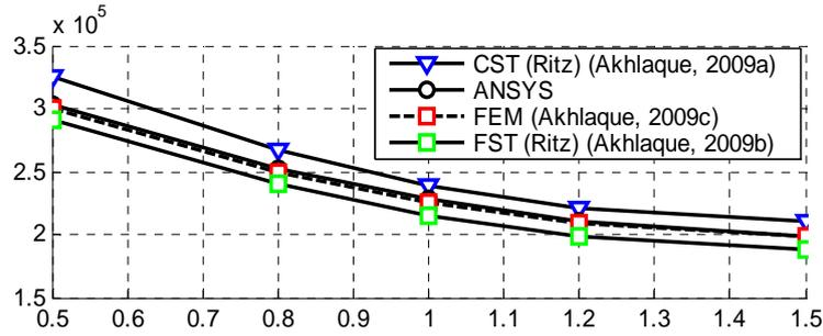
Figure 6: Variation of critical buckling load with the radius for the clamped hybrid laminate with LC<sub>1</sub> lay-up configuration.
