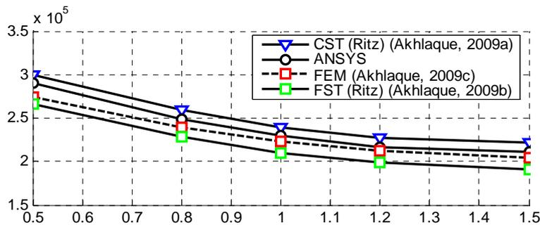
Figure 8: Variations of critical buckling load with the change of radius for the clamped hybrid laminate with LC<sub>3</sub> lay-up configuration.
