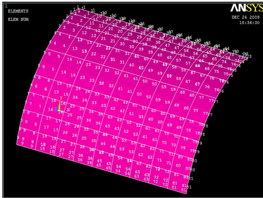
Figure 2: Finite element mesh for the cylindrical composite plate.
