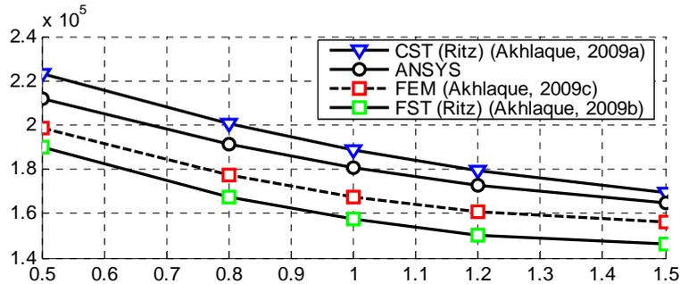
Figure 7: Variation of critical buckling load with the radius for the clamped hybrid laminate with LC<sub>2</sub> lay-up configuration.
