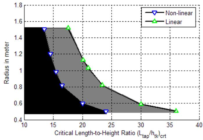
Figure 5: The effect of the radius of the tapered curved composite plate on the critical length-to-height ratio.
