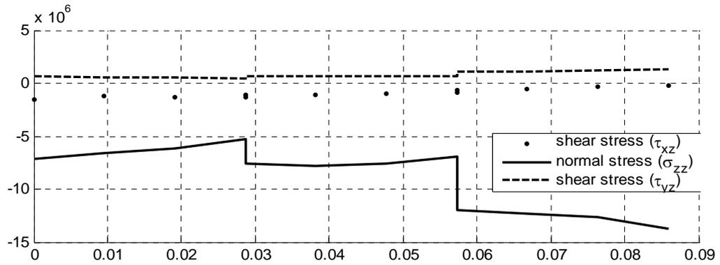
Figure 4: The stresses at the top 'resin-rich layers' with lay-up configuration  $LC_1$  and the taper configuration for the taper angle of 1 degree.
