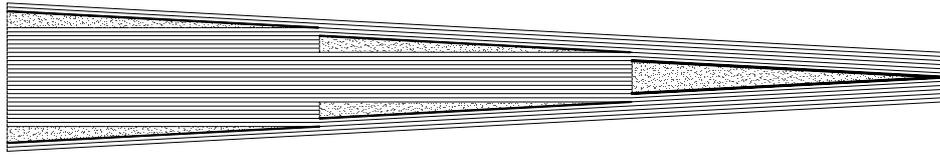
Figure 3: Longitudinal cross-section of the taper configuration with thin resin-rich layers.
