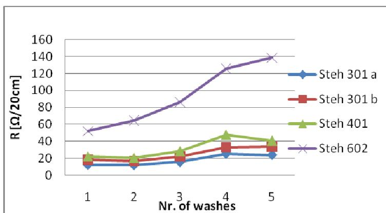
**Figure 2.**Electrical resistance of the conductive yarn after 5 washes
