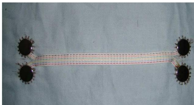
**Figure 5.** Connection with press studs
