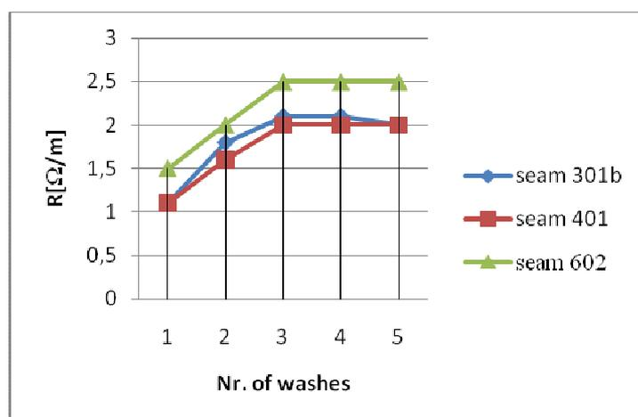
**Figure 3.** Electrical resistance of the conductive wire after 5 washes
