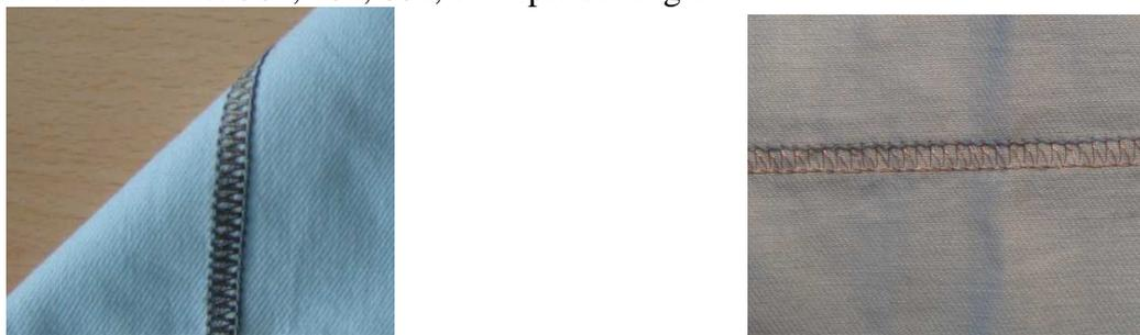
**Figure 1.** Cover stitch 602 a) stitch formed by a conductive thread, b) stitch made of copper wire
