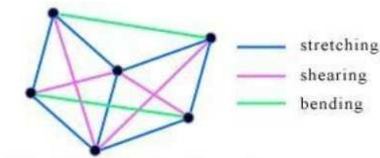
**Figure 3** : The mass-spring model [2]
