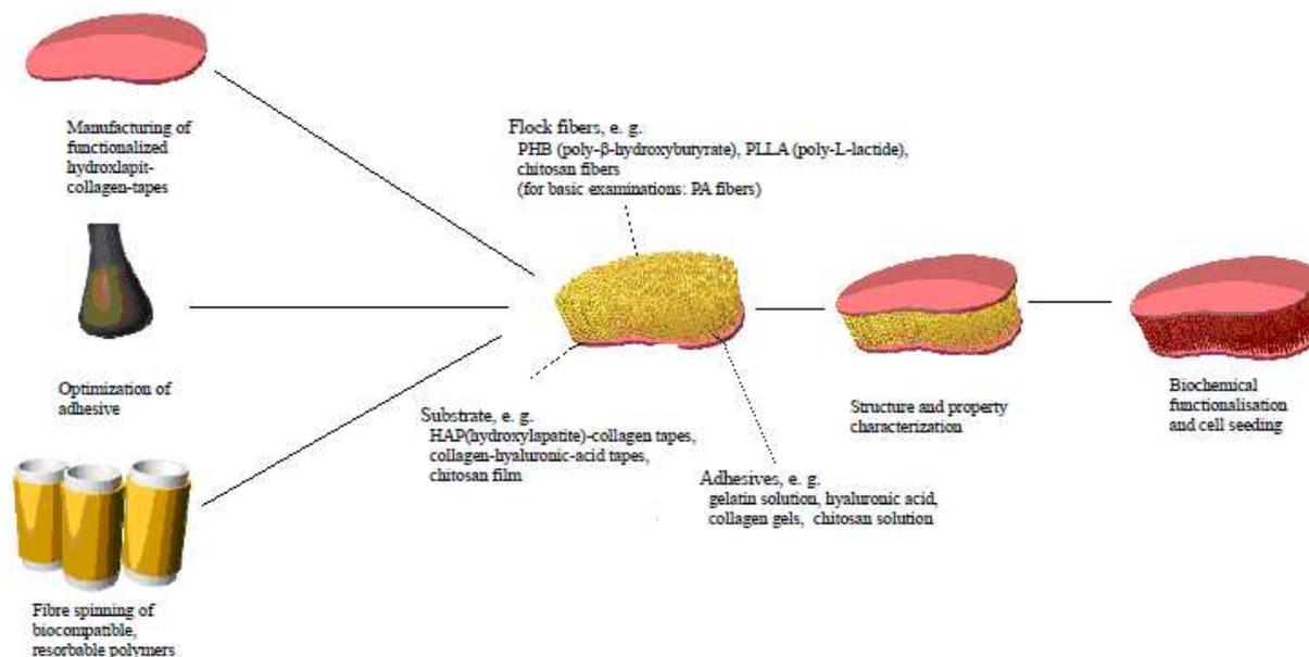
**Figure 7.** The main scheme of a flock scaffold
