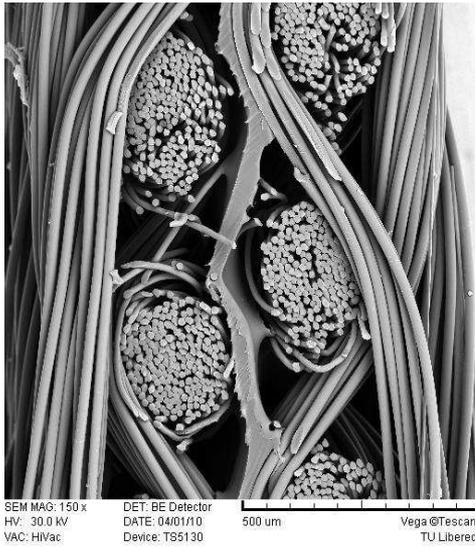
**Figure 4.** Untreated polyester fabrics bonded by polyethylene foil
