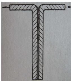
Figure 1. Form of joint for testing of adhesion by Lab Test
