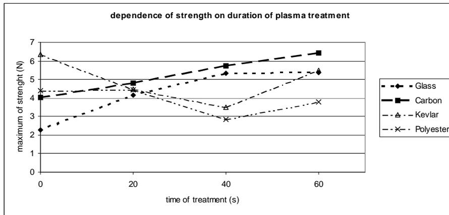
**Figure 6.** Dependence of strength on duration of plasma treatment
