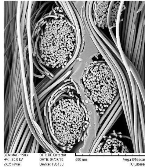
**Figure 5.** Polyester fabrics treated by plasma for 20s bonded by polyethylene foil
