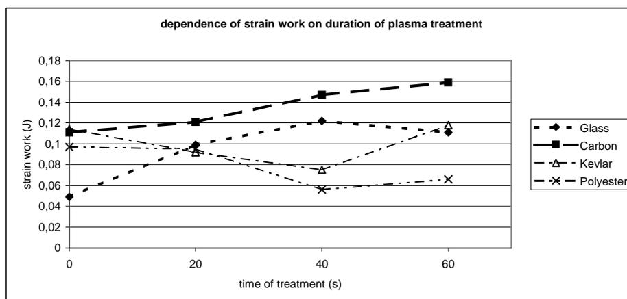
**Figure 8.** Dependence of strain work on duration of plasma treatment
