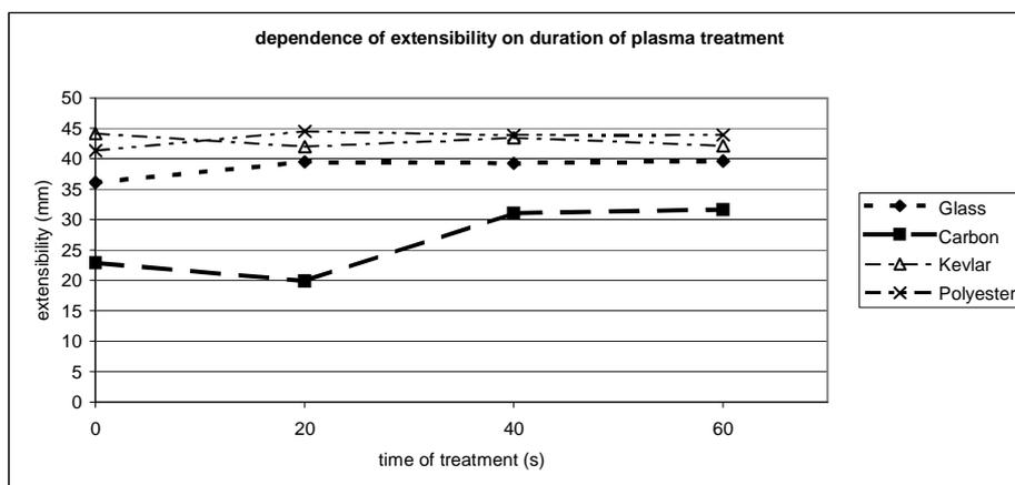
**Figure 7.** Dependence of extensibility on duration of plasma treatment
