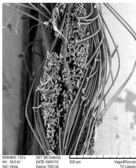
Figure 2. Untreated Kevlar fabrics bonded by polyethylene foil
