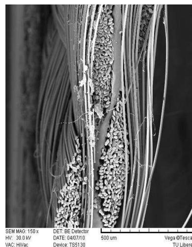
Figure 3. Kevlar fabrics treated by plasma for 40s bonded by polyethylene foil
