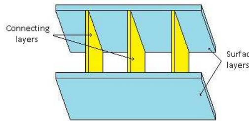
**Figure 1.** Principle of sandwich fabrics
