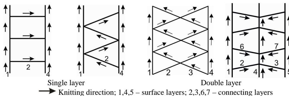
**Figure 2.1** Sandwich structures with one or two connecting layers
