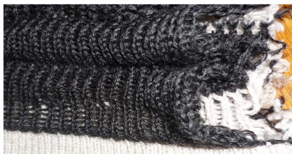
**Figure 4.3.** Sandwich structure with two binding layers
