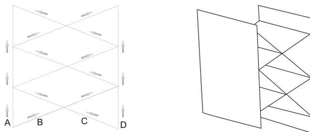
**Figure 4.1.** Principle of sandwich structure with two connecting layers
