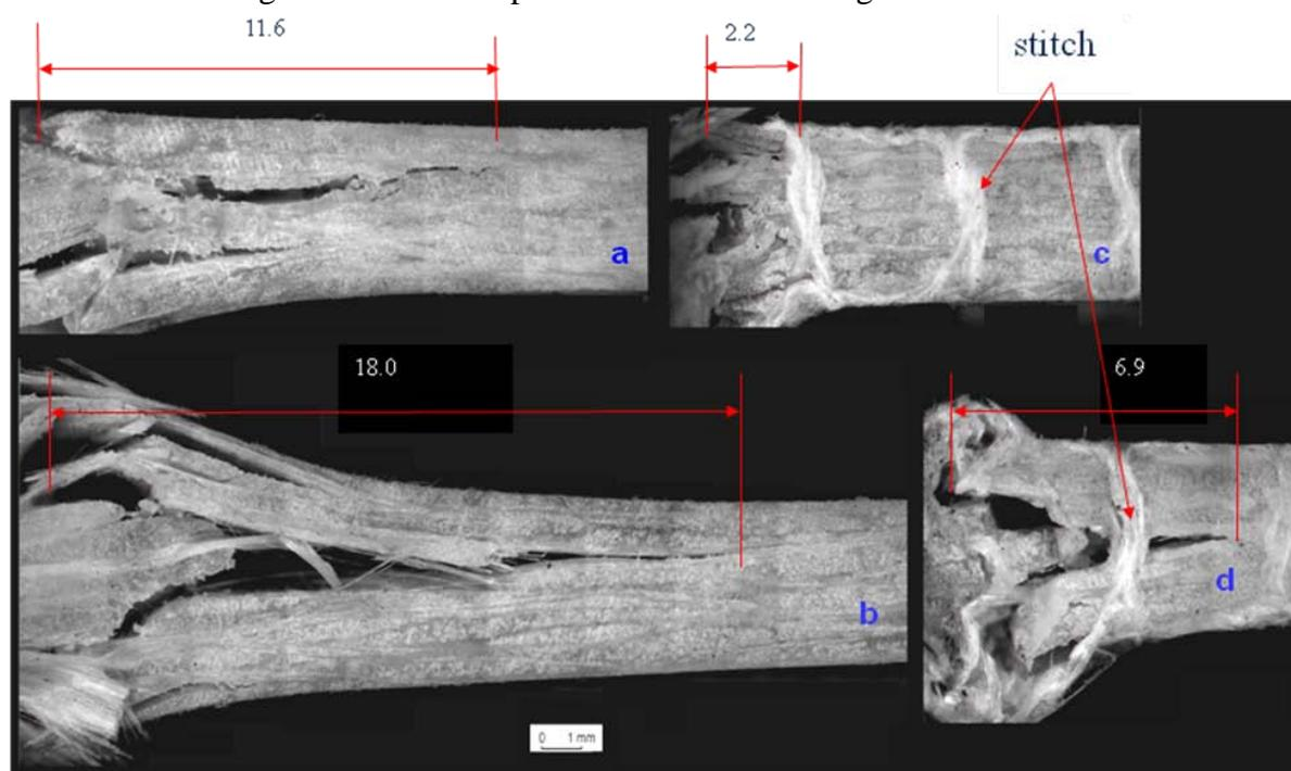
**Figure 5.** Light microscope photos of specimens after impact tests: (a) +20°C, unstitched, (b) -20°C, unstitched, (c) +20°C, stitched specimen with sewing thread GF 40, (d) -20°C, stitched specimen with sewing thread GF 50
