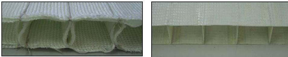
**Figure 2.** Spacer preform with uniform wall thickness and rectangular cross section made of multilayer knitted structure, textile (left) and composite (right)
