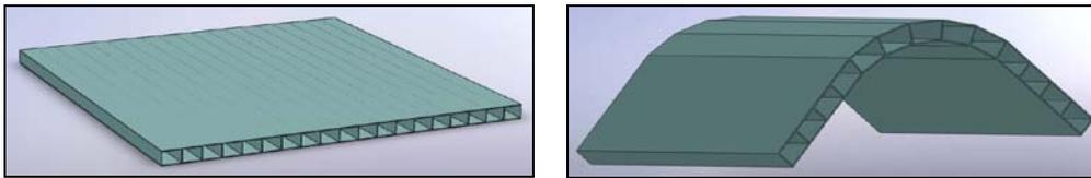
**Figure 1.** Schematic view of a flat (left) and a curved (right) spacer preform (uniform wall thickness)
