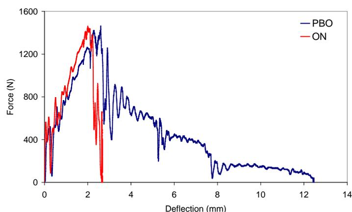
**Figure 4.** Force-deflection curves of an unstitched specimen (ON) and a stitched specimen (PBO) including PBO sewing thread at room temperature (20°C)
