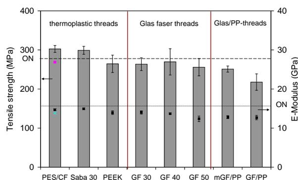
**Figure 3.** Effect of sewing threads on tensile strength and modulus of unstitched specimens and 0° stitched specimens, ON for unstitched specimen in dot line. Error bars represent standard deviations
