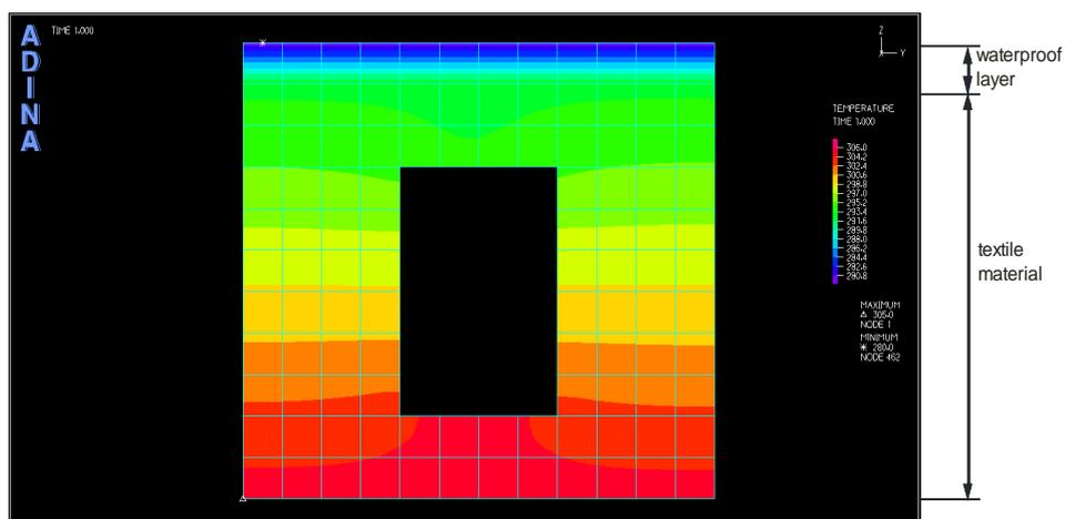
Figure 6a. Distribution of temperature for  $t=20\text{s}$
