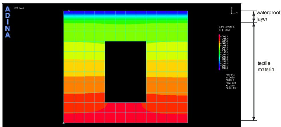
Figure 6b. Distribution of temperature for  $t=40\text{s}$
