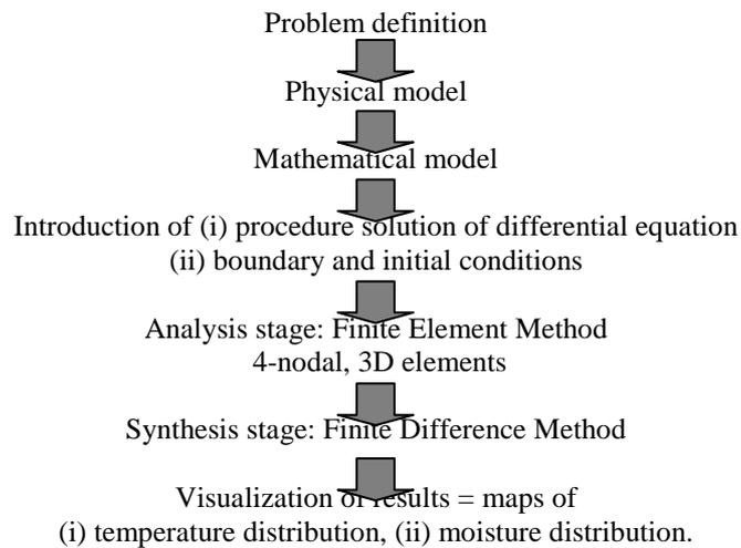
**Figure 2.** Solution strategy of the coupled heat and mass transport
