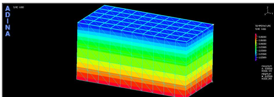
Figure 5. Distribution of water vapor concentration
