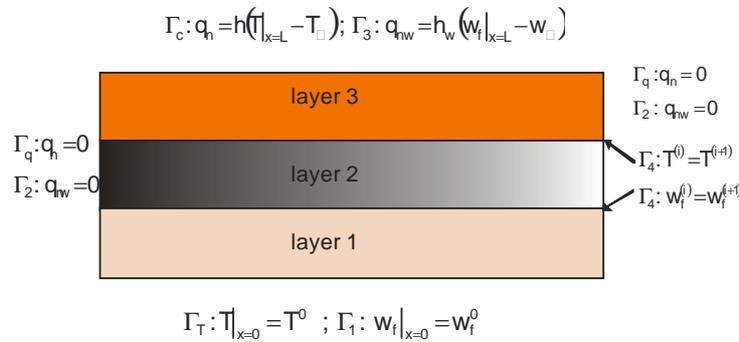
**Figure 1.** Boundary conditions of coupled heat and mass transfer
