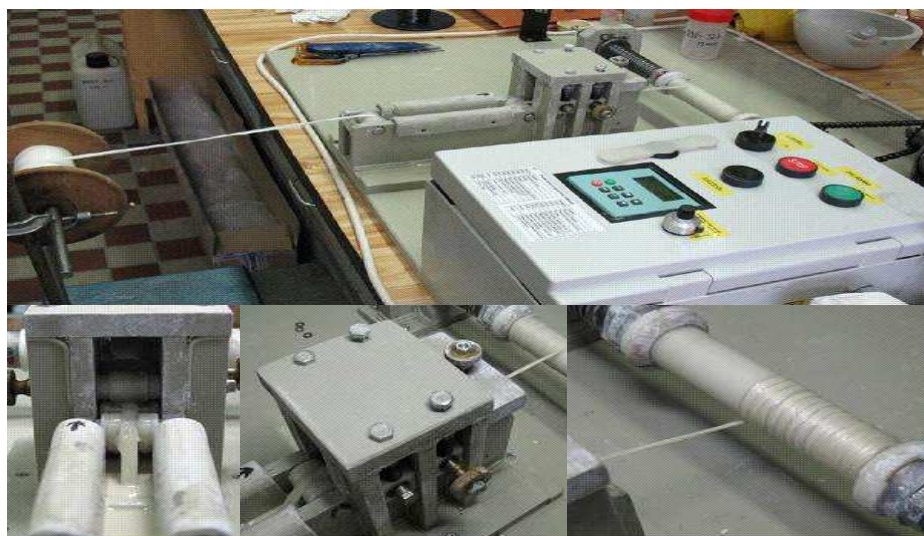
Figure 1. Home-made impregnation machine
