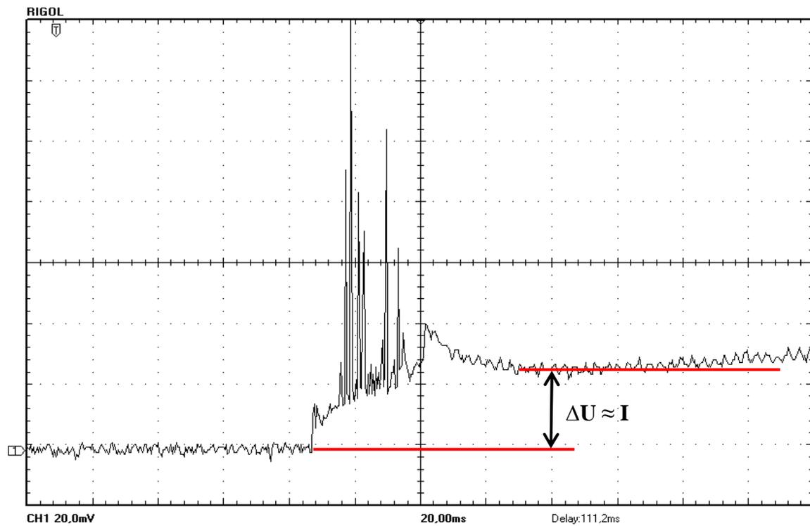
**Figure 3.** A typical record of the current during electrospinning of a spinnable polymer solution
