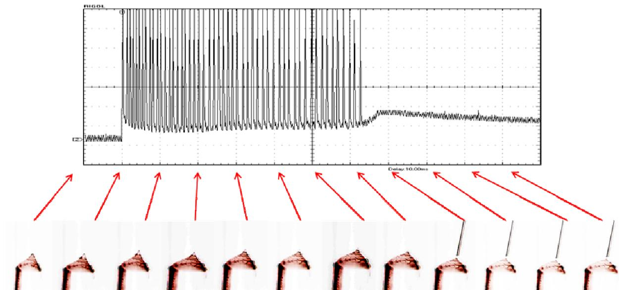
**Figure 4.** The time dependent current is compared with Taylor cone development and the jet development from high-speed camera.
