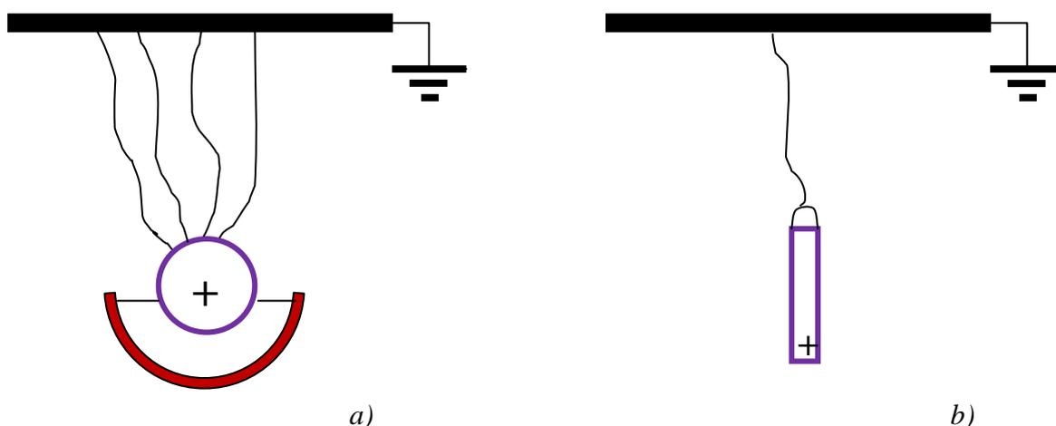
**Figure 1.** Needleless electrostatic spinners. A roller spinner (a) and a rod spinner (b)
