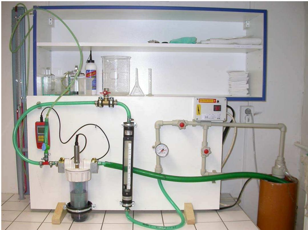
Figure. 2: Dynamic water permeability tester WPT-1
