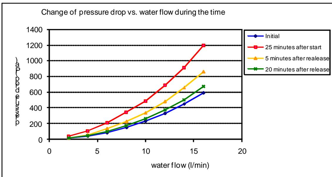
Figure. 4: Change of pressure drop of PU nanofiber layer
