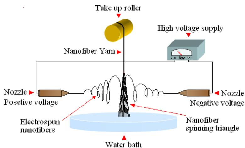
**Figure 1.** Schematic electrospinning setup to produce an open-end nanofiber yarn
