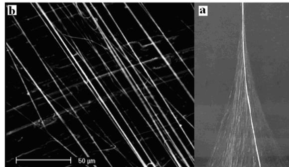
**Figure 2.** Spinning triangle image captured by a Nikon coolpix 5900 camera (a), SEM image of nanofiber orientation in the spinning triangle (b).
