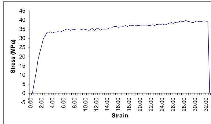
Figure 6. Typical stress-strain curve of PAN nanofiber yarn.
