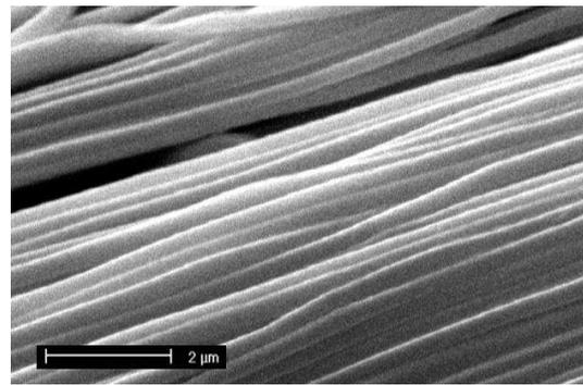
**Figure 5.** SEM image of fiber orientation in the open-end nanofiber yarn.
