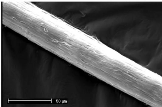
**Figure 4.** SEM image of the open-end nanofiber yarn.
