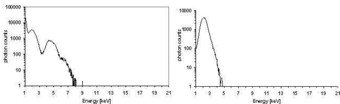
**Figure 1.** (a) Continuous energy spectra of X-ray total photon count accumulated during 150 s emitted from the end of PVA electrospinning jets recorded by the unshielded SLP X-Ray Detector. The distance between the needle and the collector was adjusted on 50 mm and the voltage was 15 kV.
