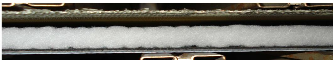
Figure 8. WNV nonwoven between compression belts (at 55 mm distance) in the thermal bonding oven
