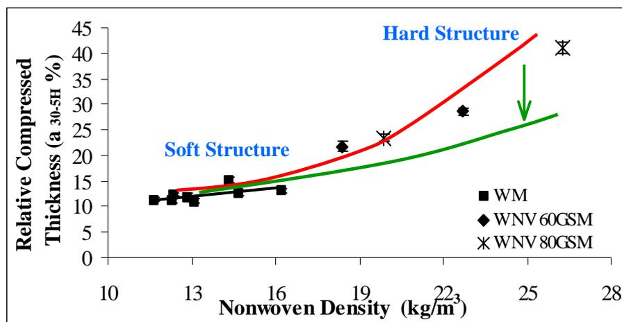
Figure 10. Effect of feeding web type and nonwoven density on RCT ( $a_{30-5H}$ )
