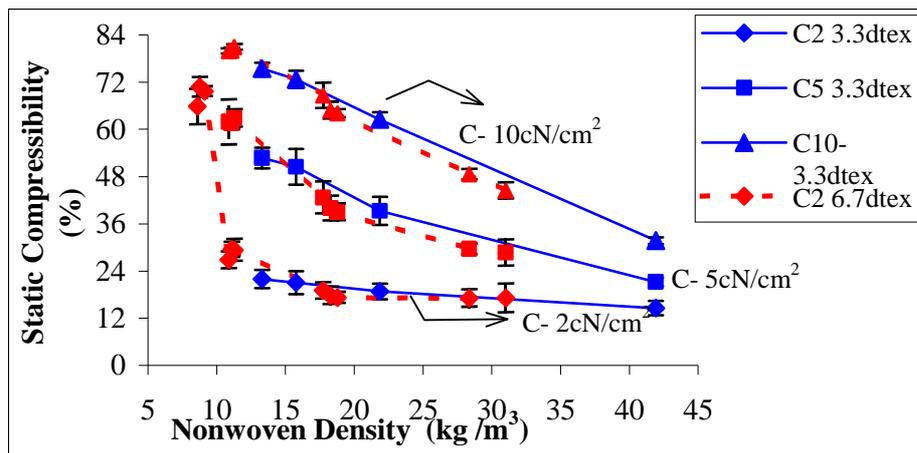
Figure 4 Effect of fiber fineness and nonwoven density on static compressibility
