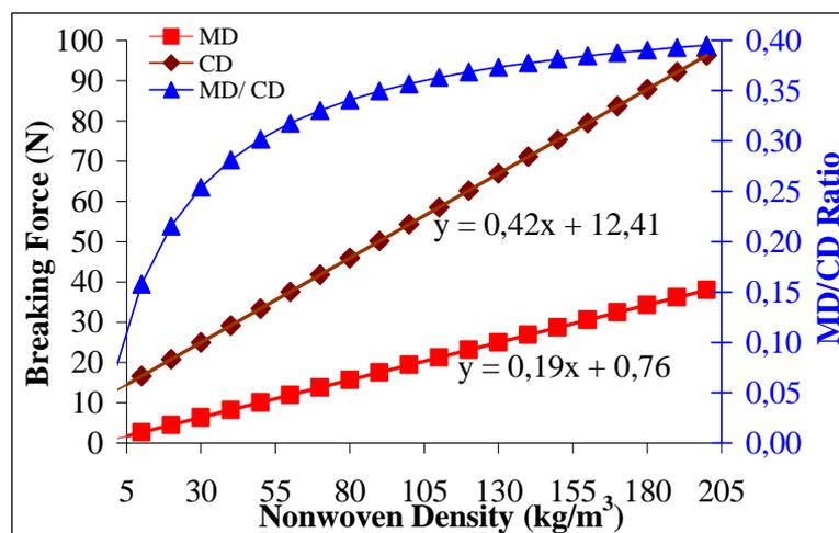
**Figure 3.** Effect of nonwoven density on tensile behavior
