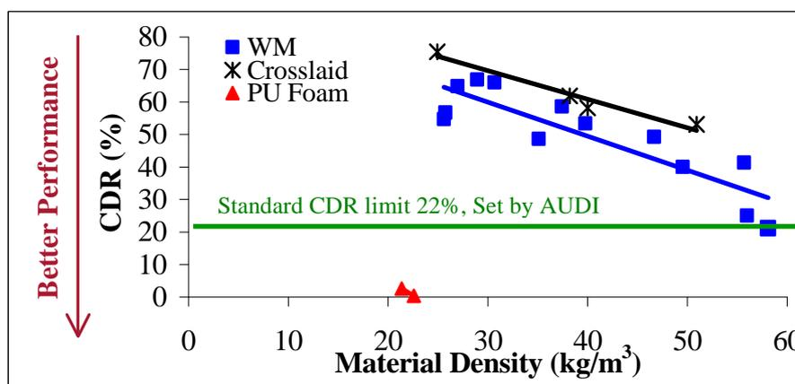
Figure 5. Effect of material density and structure on CDR [17]
