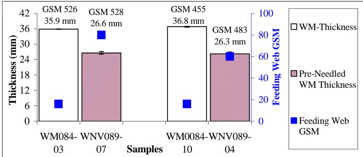
Figure 6. Effect of feeding web type on Wavemaker nonwoven thickness
