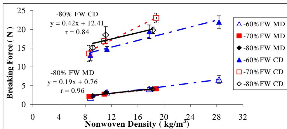
**Figure 2.** Effect of FWS and nonwoven density on tensile strength (FWS lagging to working wheel speed, each set of WM nonwovens belong to a particular thickness for same the GSM)
