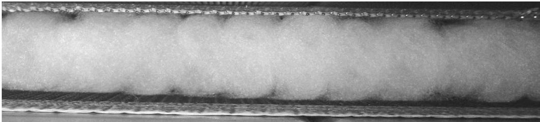
Figure 7. WNV nonwoven between compression belts (at 55 mm distance) before entering in thermal oven
