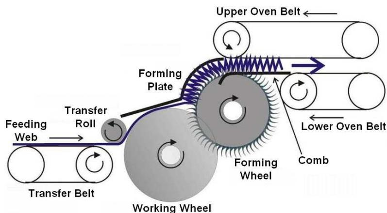
Figure 1. Wavemaker working principle, Set-up at ITV Denkendorf
