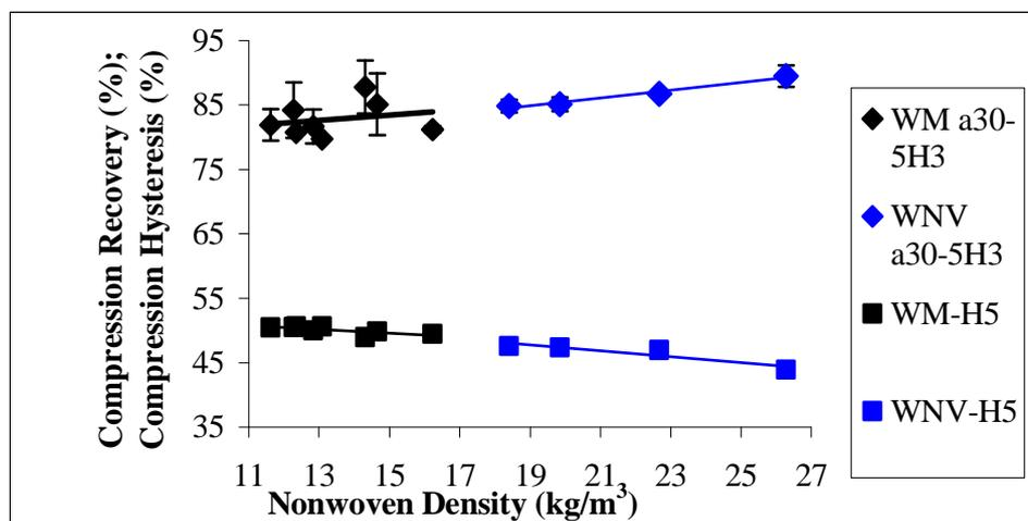
Figure 11. Effect of feeding web type and nonwoven density on dynamic compression recovery and hysteresis
