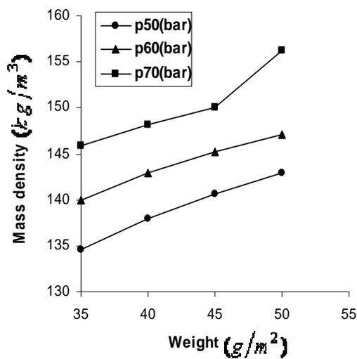
Figure 3. Changes in mass density with increasing of basis weight and water jet pressure
