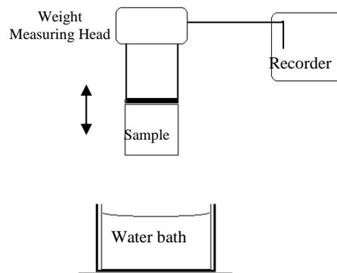
**Figure 1.** . The mechanism of measurement method for water retention
