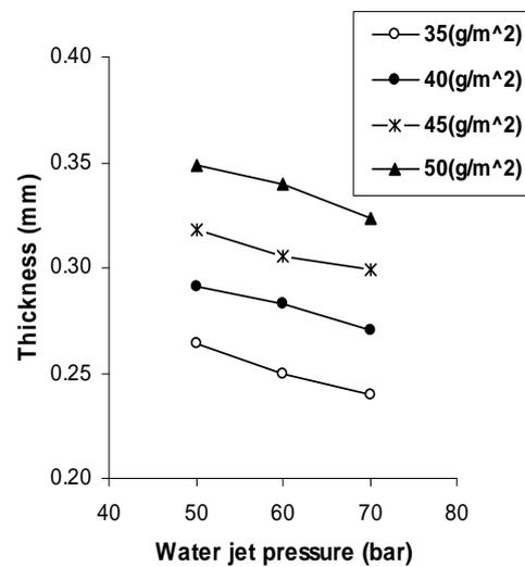
Figure 4. Changes in thickness with increasing of basis weight and water jet pressure
