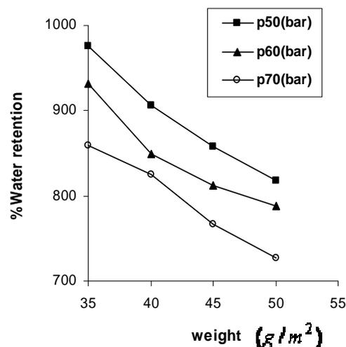
Figure 6. Changes of water retention percent with increasing of basis weight and water jet pressure
