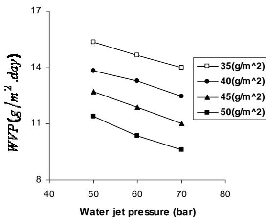
Figure 5. Effect of water jet pressure and basis weight on WVP of samples
