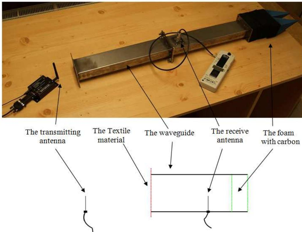
**Figure 4** The measurement device
