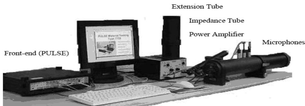
**Figure 9:** System configuration of acoustical material testing using two-microphone method
