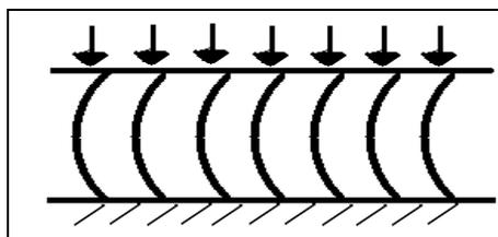
Figure 2. Monofilaments as the curved bars in compression
