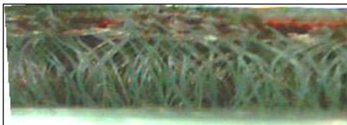
Figure 4.Spacer fabric in weft direction
