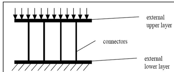
Figure 1. Monofilaments as the vertical bars in compression [5]
