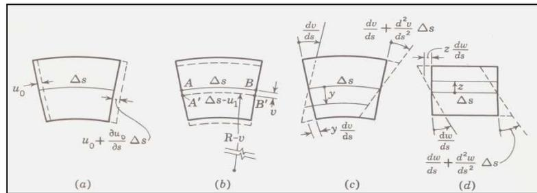
Figure 3. Deformation of a curved bar element[6]
