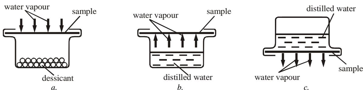
**Figure 1.** Schemes for measuring vapor permeability by “cup method” (ASTM E96):
