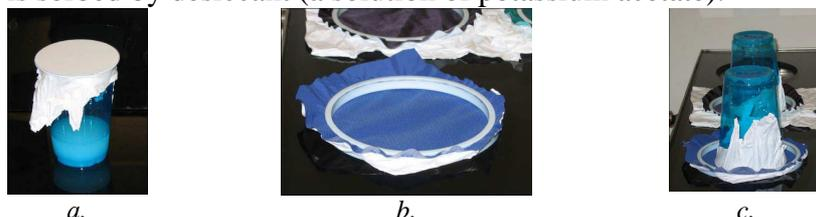
**Figure 2.** Scheme for measuring vapor permeability by “inverted desiccant method”
