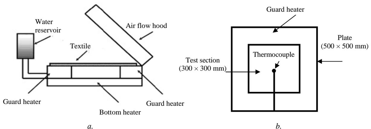
**Figure 4.** Scheme for measuring vapor permeability by “sweating hot plate” method on device SGHP-8.2 [ISO 11092 (EN 31092)]
