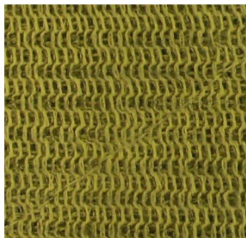
Fig 10. Detail of Kevlar-steel wire knitting
