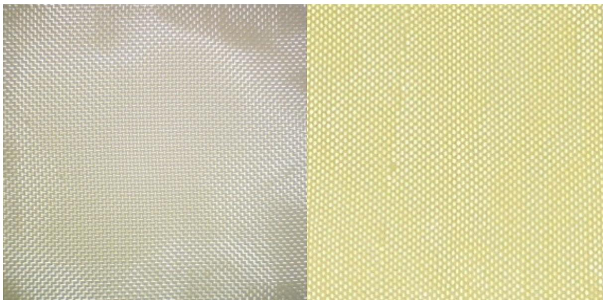
**Fig 11.** Detail of ballistic nylon fabric**Fig 12.** Detail of Kevlar fabric
