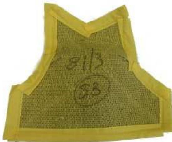
Fig 8. Knife and arrow protection
