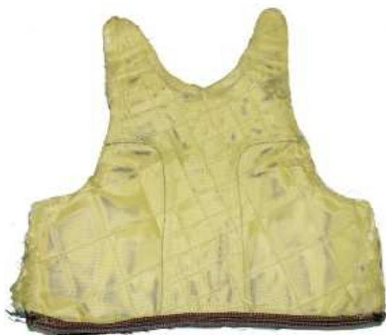
Fig 7. 26 Kevlar layers sewn together
