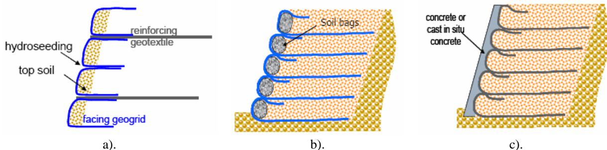
Figure 3. The design method recommended for retaining walls reinforced with geo-textile
