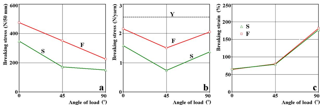
Figure 11. Example of breaking stresses and strains for knitted interlock fabric
