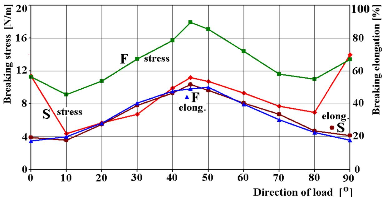
Figure 8. Breaking stresses and strains, pure cotton, finished fabric
