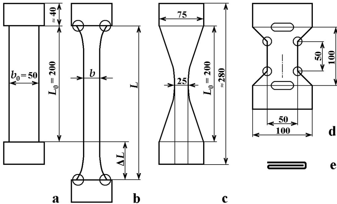
Figure 1. The main principles of measuring of fabric rupture properties
