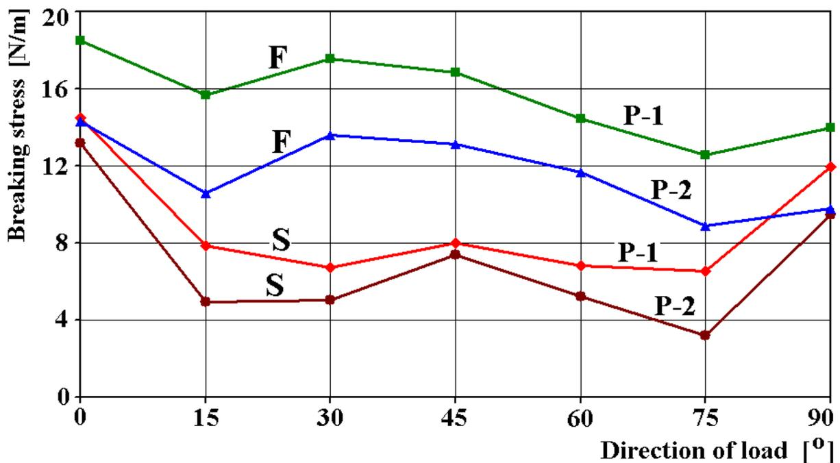
Figure 5. Anisotropy in tensile properties (fabrics P-1 and P-2)
