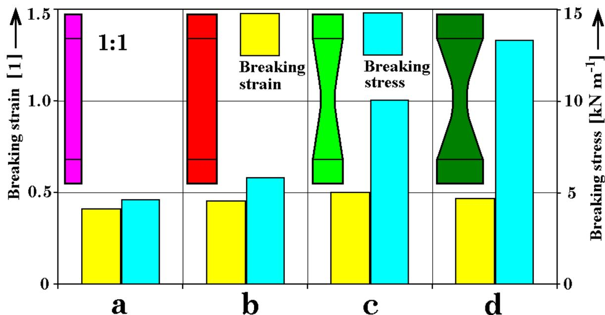
Figure 3. Influence of sample shapes on breaking stress and strain
