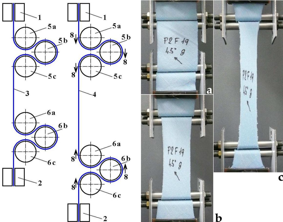
Figure 2. The principle of tensile properties measuring with the use of capstan friction
