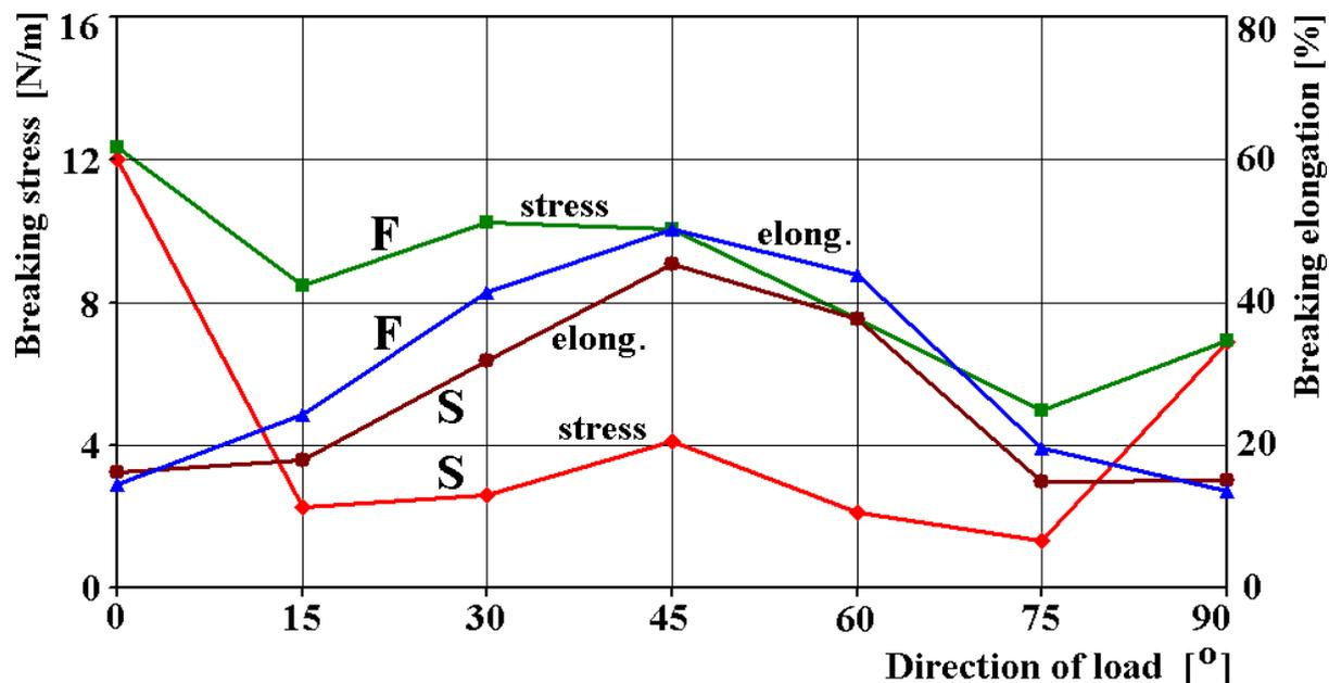
Figure 6. Breaking stresses and strains, polypropylene 35 % and cotton 65 % blend
