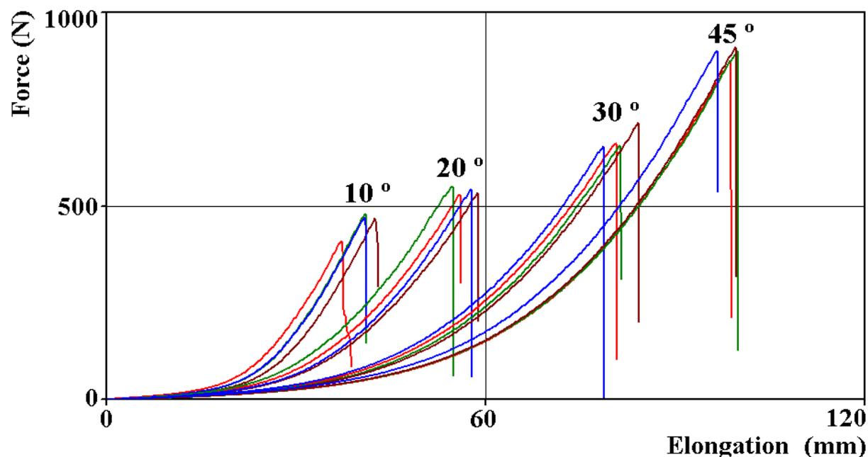
Figure 9. Examples of stress-strain curves – F (friction) tests
