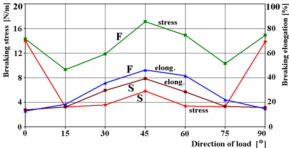
Figure 7. Breaking stresses and strains, pure cotton, gray fabric
