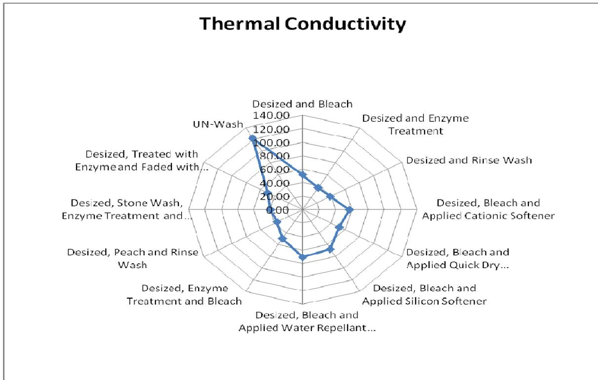
**Figure 1** The effect of finishing on thermal conductivity of denim fabrics
