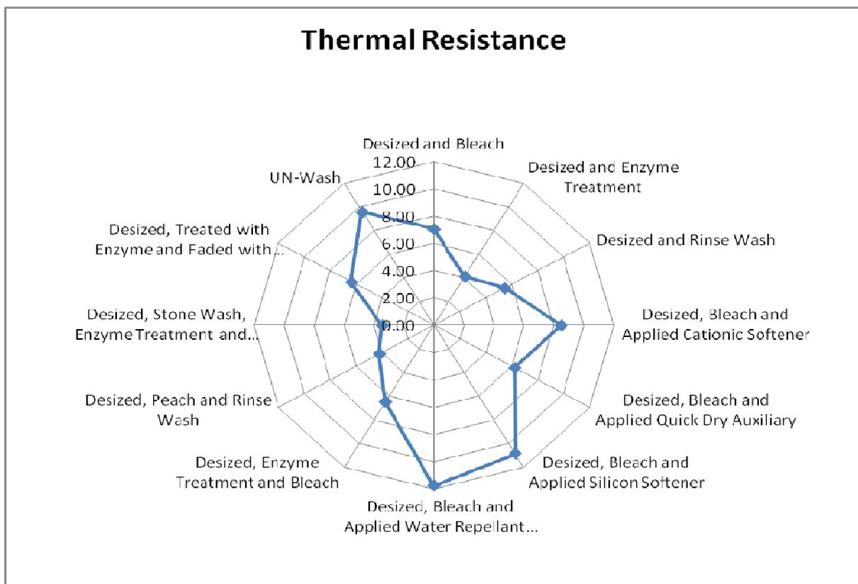
**Figure 2** The effect of finishing on thermal resistance of denim fabrics
