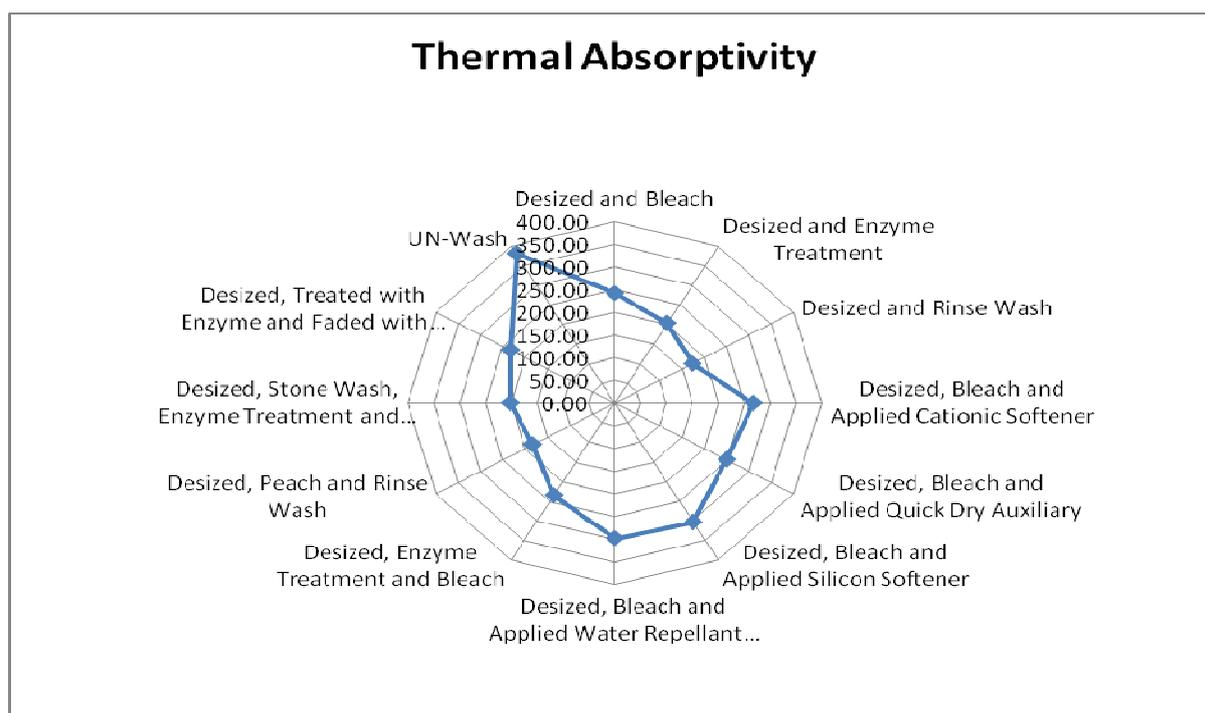
**Figure 3** The effect of finishing on thermal absorbtivity of denim fabrics
