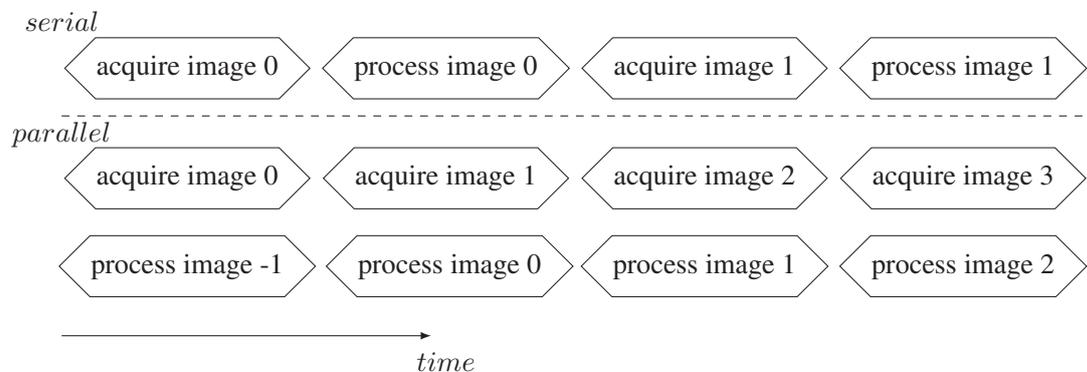
Fig. 6: Image acquisition and analysis cycle.
