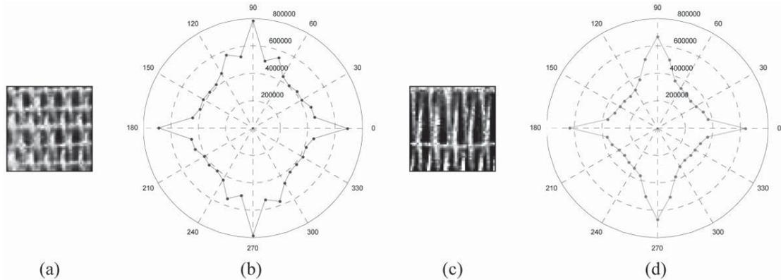
Fig. 1: (a) Window with non-defective area, (c) window with defective area, (b),(d) polar plots of  $S_\alpha$  in 10 degree step.
