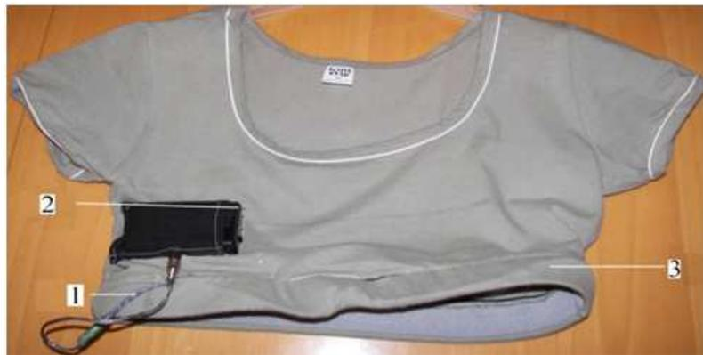
**Figure 3.** Prototype of a t-shirt with a piezoelectric sensor
