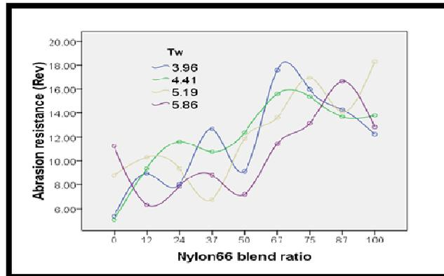
Figure 8. Effect of nylon66 blend ratio on the abrasion resistance of nylon66/cotton rotor yarn
