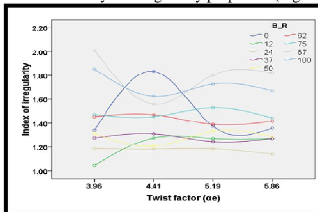
**Figure 4.** Effect of twist factor on the Index of irregularity of nylon66/cotton rotor spun yarn.
