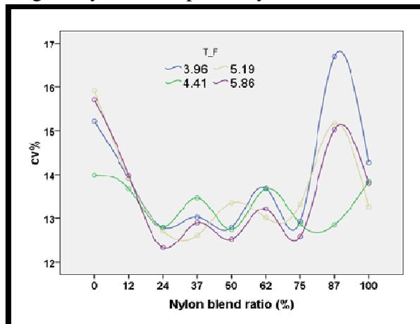
**Figure 2.** Effect of nylon66 blend ratio on nylon66/cotton blended rotor spun yarn irregularity (CV%).
