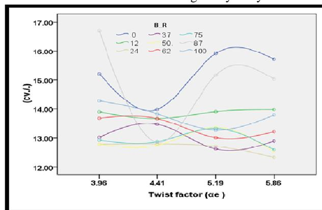
**Figure 5.** Effect of twist factor on nylon66/cotton blended rotor spun yarn irregularity (CV%).
