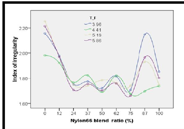
**Figure 3.** Effect of nylon66 blend ratio on nylon66/cotton blended rotor spun yarn irregularity index (I).
