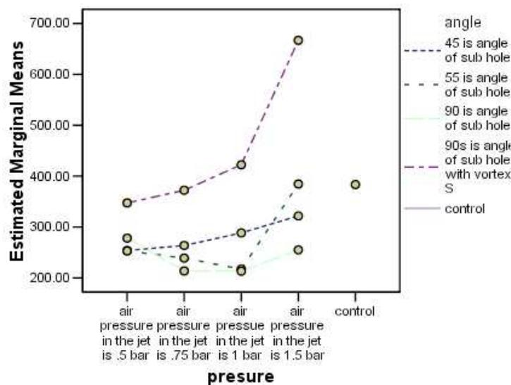
Figure 3. Rotor-spun yarn hairiness at different take-up air-nozzle types and air pressure values
