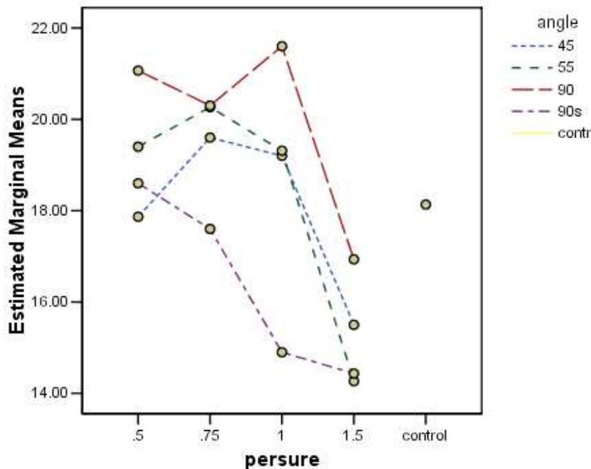
Figure 6. Rotor-spun yarn tensile elongation (%) at different take-up air-nozzle types and air pressure values
