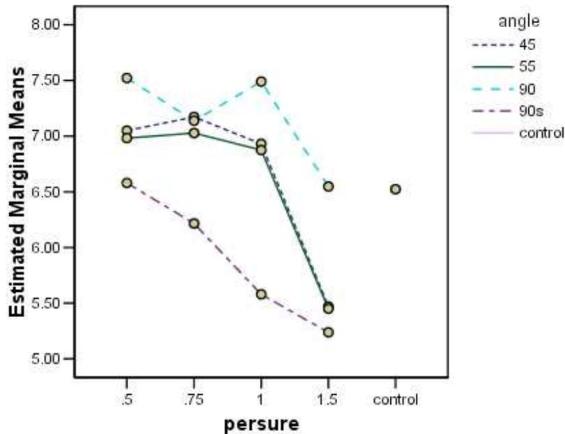
Figure 5. Rotor-spun yarn tensile strength (cN/tex) at different take-up air-nozzle types and air pressure values
