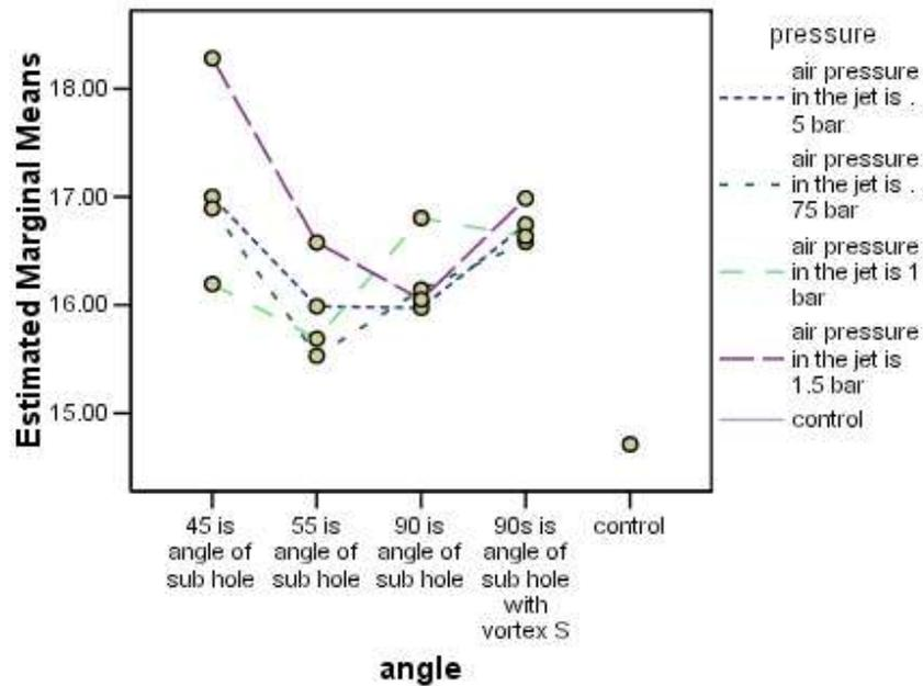
Figure 3. Rotor-spun yarn irregularity (CV%) at different take-up air-nozzle types and air pressure values
