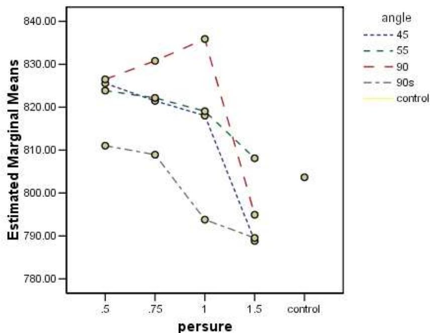
Figure 3. Rotor-spun yarn twist (T.P.M) at different take-up air-nozzle types and air pressure values
