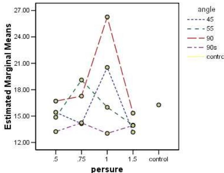
Figure 4. Rotor-spun yarn abrasion resistance at different take-up air-nozzle types and air pressure values
