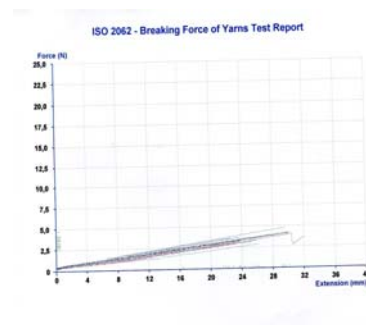
Figure.6 Strain diagram of yarn in loop
