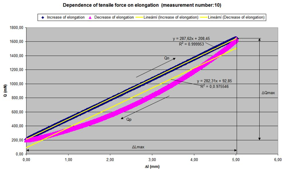
**Figure 5:** Dependence of tensile force on elongation (measuring No.10)
