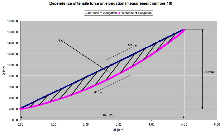
**Figure 4:** Dependence of tensile force on elongation during extension and loosening of threads
