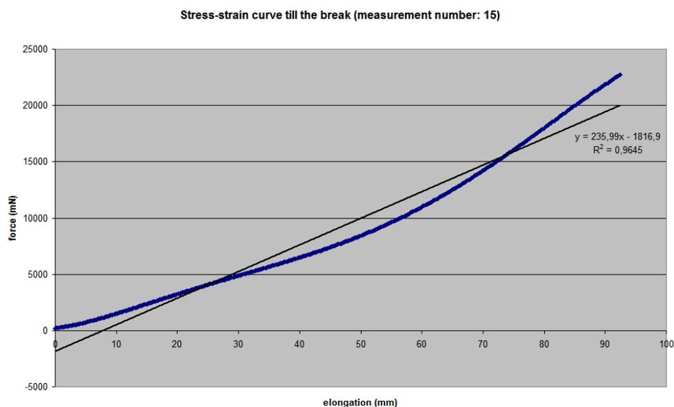
**Figure 2:** Stress-strain curve and its regression straight line
