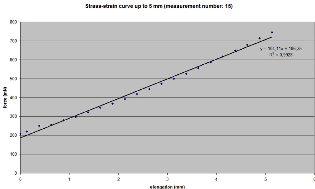
**Figure 3:** Stress-strain curve up to 5 mm and its regression straight line
