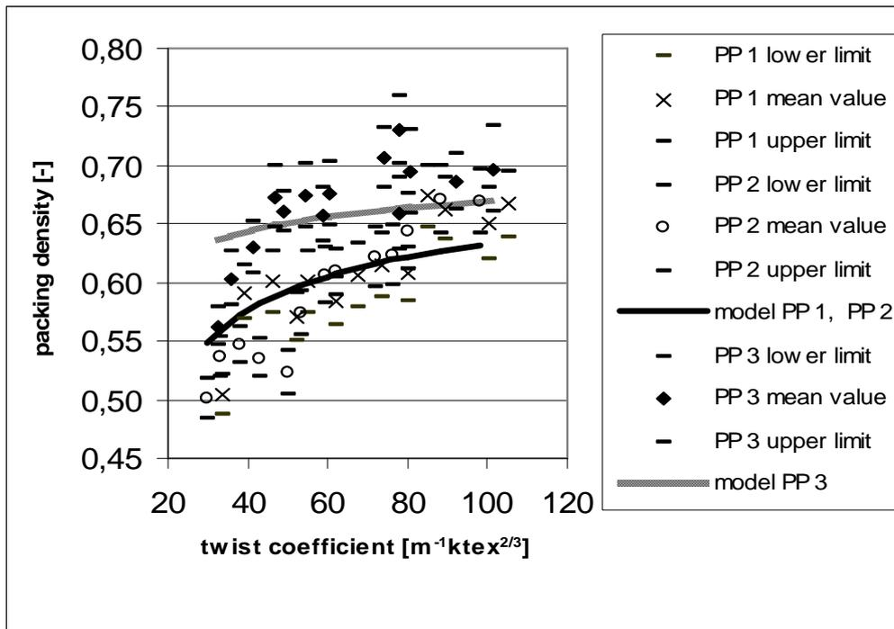
Fig. 1 Yarn packing density as function of twist coefficient
