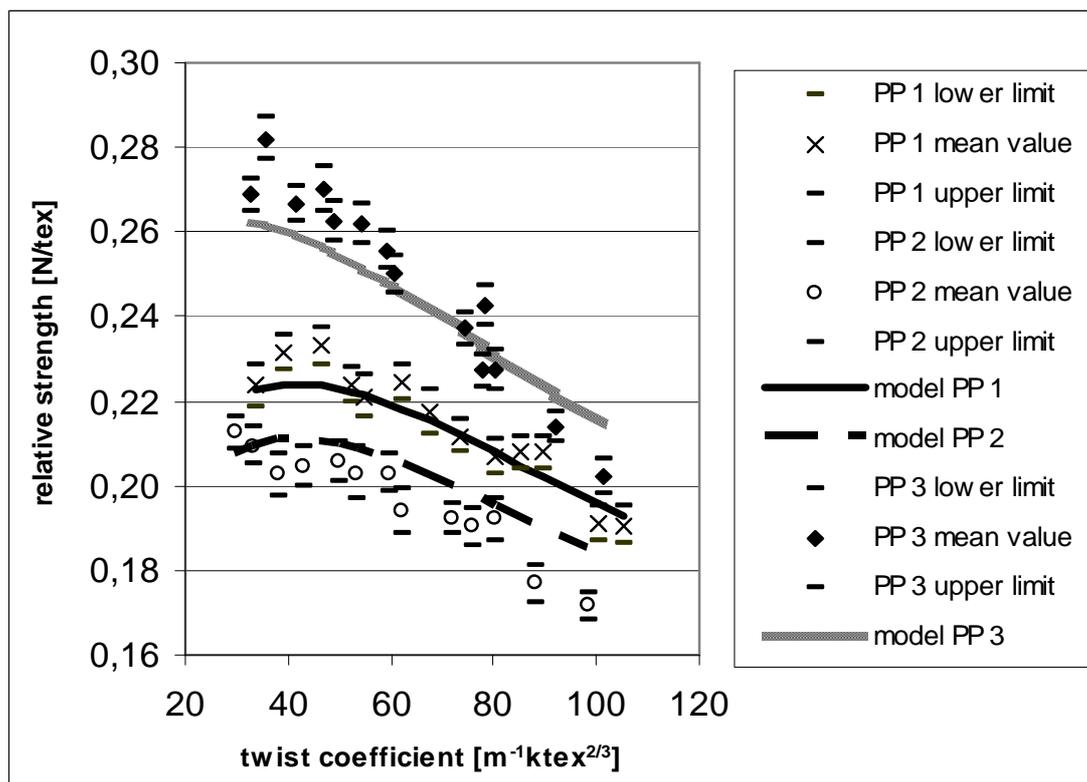
Fig. 3 Yarn strength as function of twist coefficient
