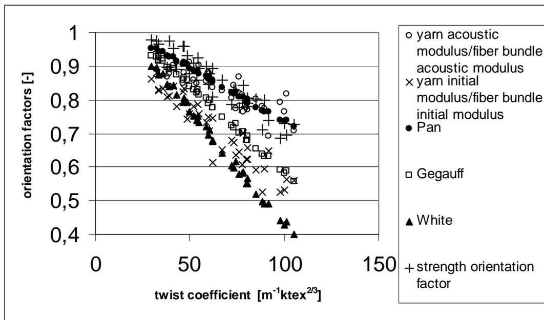
Fig. 2 Orientation factors as function of twist coefficient
