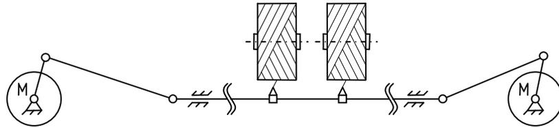
Figure 5. Double crank mechanism
