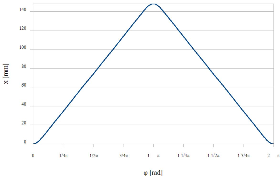
**Figure 2.** Yarn guide motion shape
