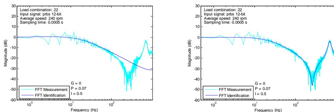
Figure 7. Bode plot of servo drive and its identification
