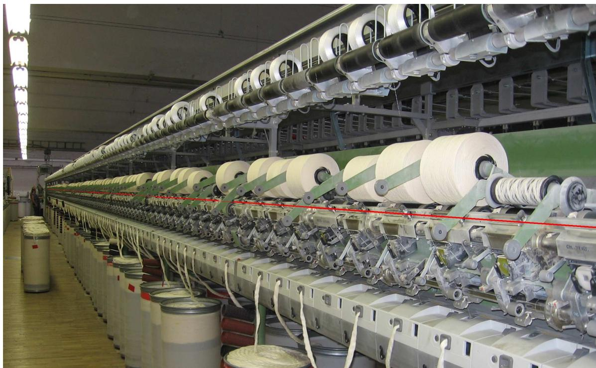
**Figure 1.** Rotor spinning machine
