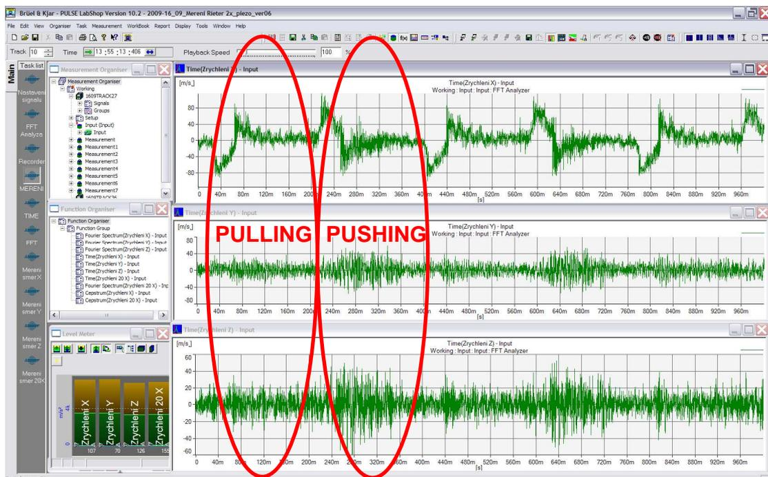
Figure 4. Measurement of vibrations – pulling and pushing phase
