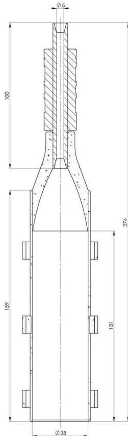
Fig. 3: Diagram of the separator
