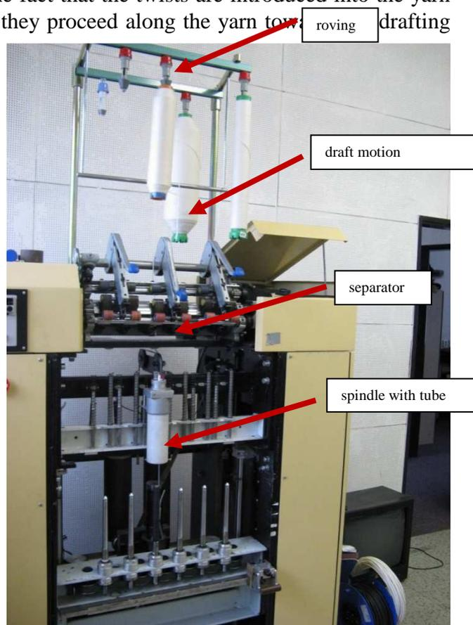
Fig. 4: Functional model of loop spinning
