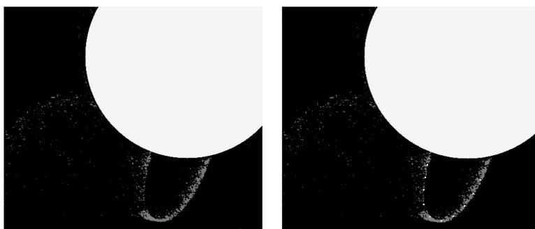
**Fig. 6:** On the left, the adjusted snapshot intended for the analysis, on the right, the established trajectory of the yarn
