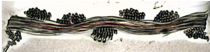
Figure 7. Image of binding wave coordinates in transverse cross section in woven fabric (PES threads)
