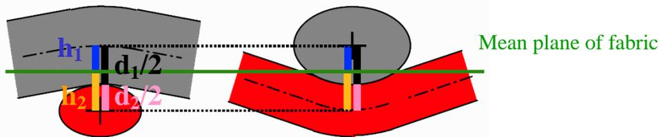
Figure 4. Description of heights of binding wave and yarn diameters in binding wave
