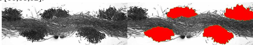
Figure 8. Real cross section (image analysis Software NIS Elements) – real shape
