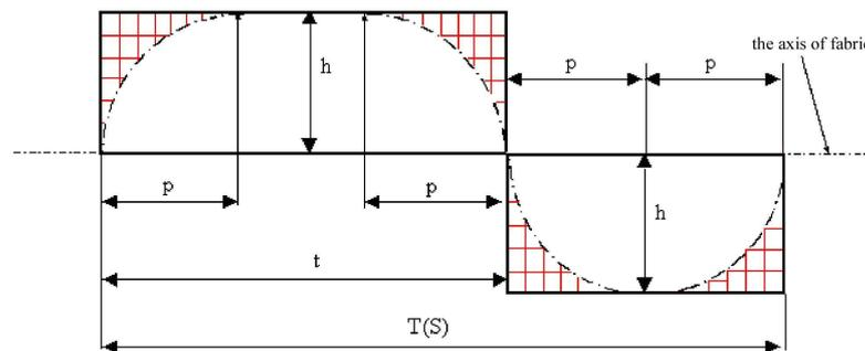
Figure 14. Description of binding wave in fabric for Fourier mathematical model
