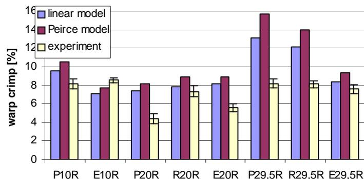
**Figure 15.** Comparison of theoretical and experimental warp crimp
