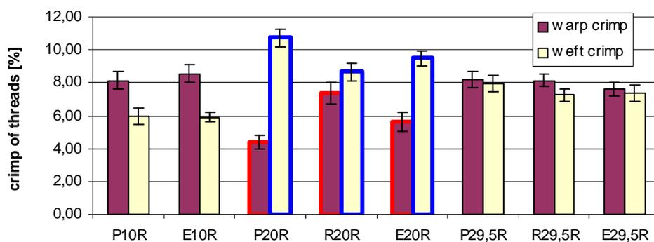
Figure 18. Comparison of warp and weft crimp – experimental values
