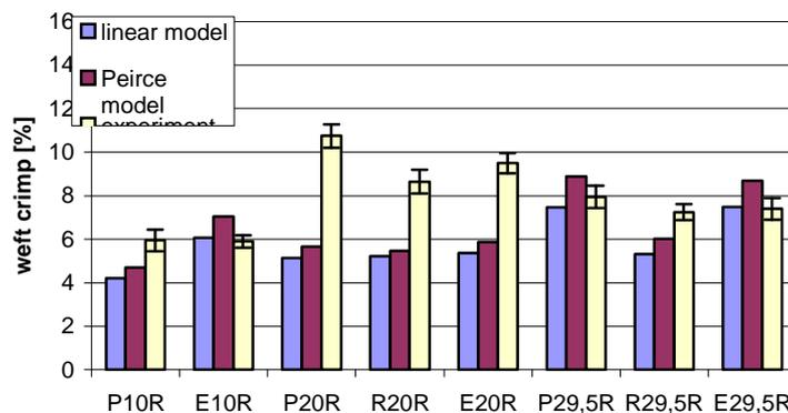
**Figure 16.** Comparison of theoretical and experimental weft crimp
