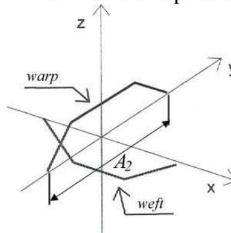
Figure 10. Linear model for description of binding wave
