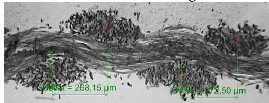
Figure 3. Evaluation of warp distances in transverse cross section
