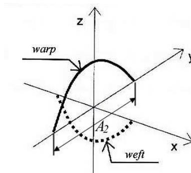
Figure 12. Hyperbolic model for description of binding wave
