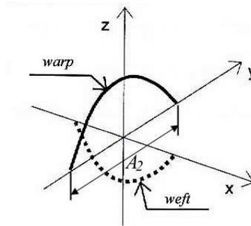
Figure 11. Parabolic model for description of binding wave
