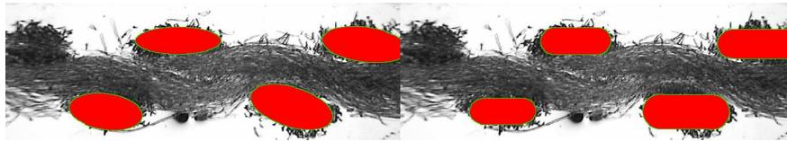
Figure 9. Substitution of real yarn in cross-section – ellipse, Kemp model
