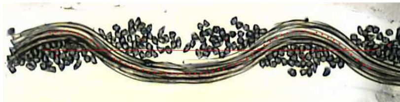
Figure 6. Image of binding wave coordinates in longitudinal cross section in woven fabric (PES threads)
