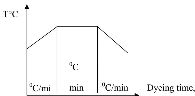
**Fig. 2.** Dyeing diagram of cotton knitted fabrics with direct and disperse dyes
