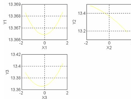
Fig. 17. The variation of knitted fabrics loop length depending on dyeing time, temperature and pH
