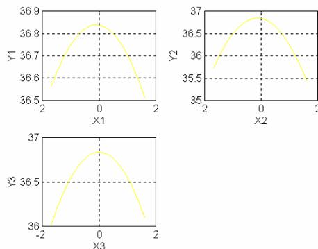
**Figure. 3.** The variation of knitted fabrics wale density depending on dyeing time, temperature and pH
