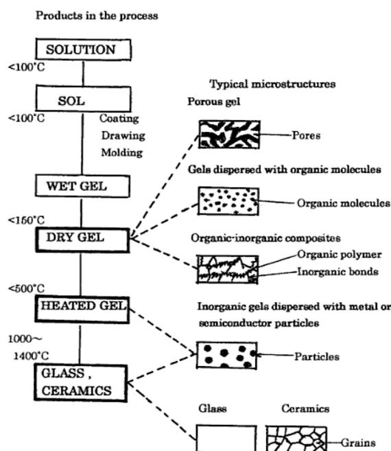
**Figure 1.** Steps of the sol-gel processing of materials and examples of the microstructure of final products. Bold-lined rectangles show possible final of the sol-gel method [3].
