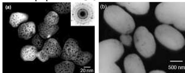
Fig. 2 TEM images of nano (a) and micro (b) particles of the as-prepared  $\alpha$ -Fe<sub>2</sub>O<sub>3</sub>.
