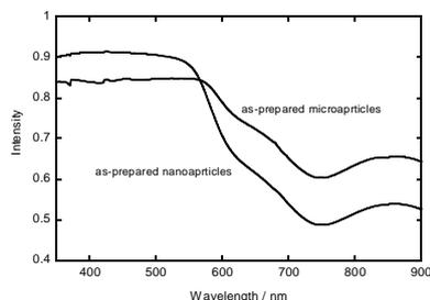
Fig. 5 UV-visible diffusion spectra for nano- and micro particles of  $\alpha$ -Fe<sub>2</sub>O<sub>3</sub>.
