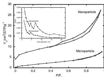
Fig. 4 Nitrogen adsorption isotherm of nano- and micro particles of  $\alpha$ -Fe<sub>2</sub>O<sub>3</sub>.
