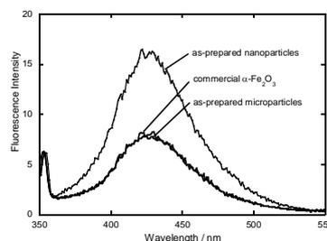
Fig. 6 Fluorescence spectra for as-prepared  $\alpha$ -Fe<sub>2</sub>O<sub>3</sub> nano-, micro-particles and commercial  $\alpha$ -Fe<sub>2</sub>O<sub>3</sub> nanoparticles.
