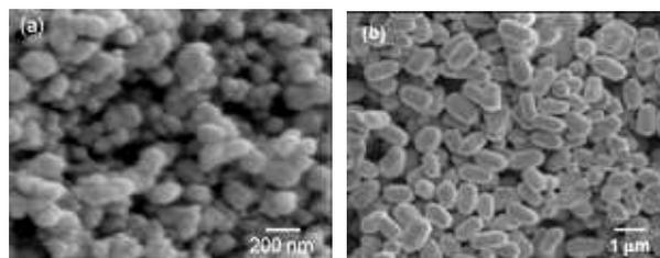
Fig. 1 SEM images of nano (a) and micro (b) particles of the as-prepared  $\alpha$ -Fe<sub>2</sub>O<sub>3</sub>.
