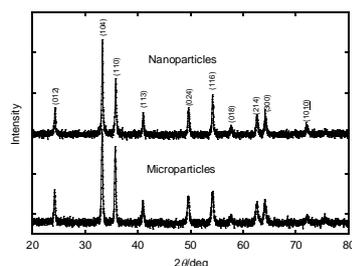
Fig. 3 XRD pattern of  $\alpha$ -Fe<sub>2</sub>O<sub>3</sub> nano and micro particles.
