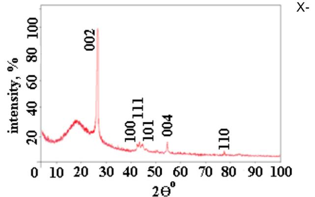
ray analysis of the dispersion of graphite products (sludge) in toluene showed that the sample contains amorphous carbon, graphite and ultra-fine diamond particles.
