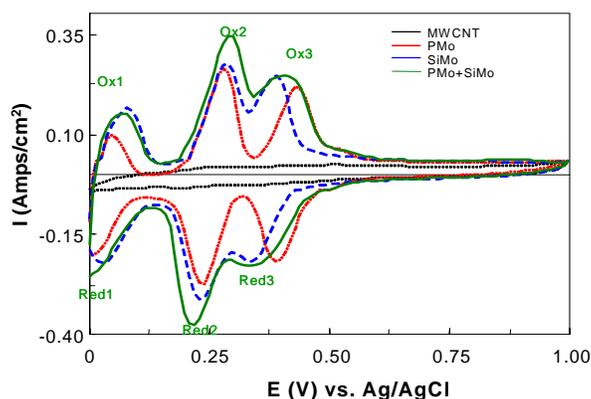
Fig.2. CV profiles of bare MWCNT, a single-layer  $\text{PMo}_{12}$  (red),  $\text{SiMo}_{12}$  (blue) coated and a dual-layer ( $\text{PMo}_{12}$  +  $\text{SiMo}_{12}$  TL) (green) coated MWCNT in 1M  $\text{H}_2\text{SO}_4$ .
