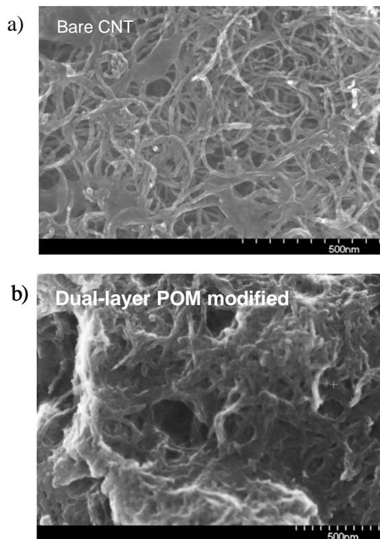
Fig.3. SEM micrographs of a) bare MWCNTs and b) POM modified MWCNTs.
