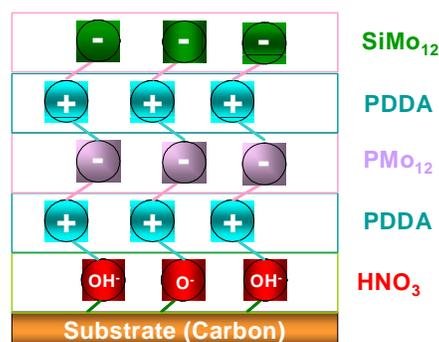
Fig. 1. A schematic diagram of LbL deposition of POM modification on CNT.
