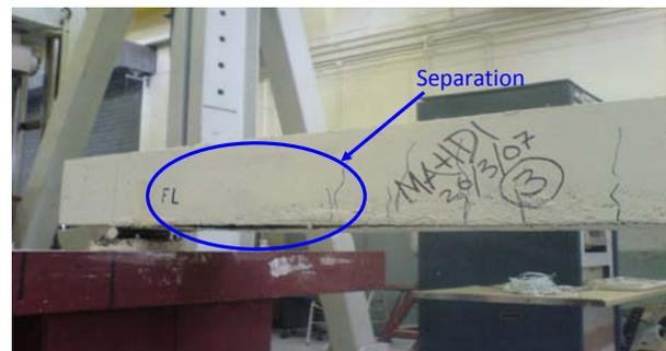
Figure 3: Bond Failure in CF sheets bonded with mortar
